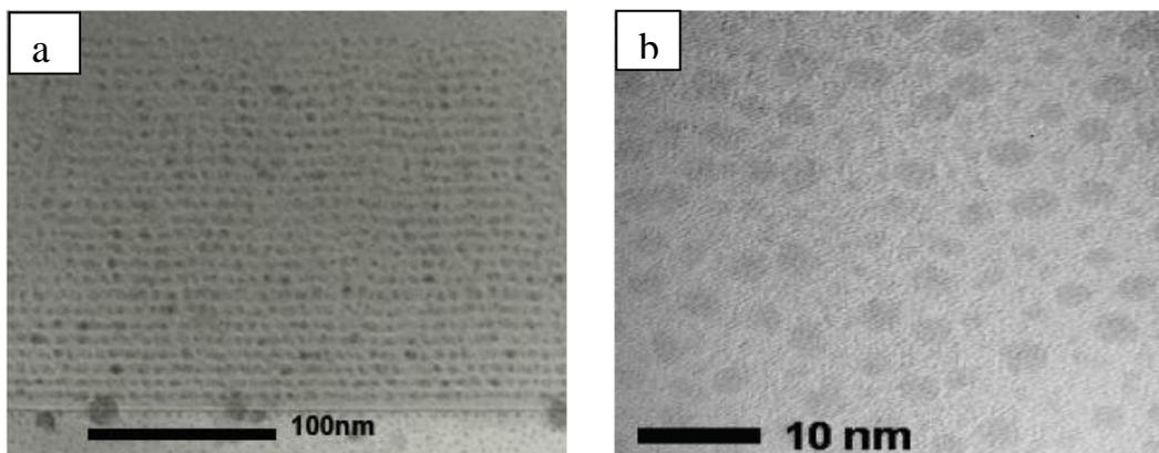
**Figure 2:** (a) Cross-sectional view TEM image of silicon quantum dot layers prepared in an oxide matrix; (b) Plan view TEM image of a single layer of silicon quantum dots showing lateral spacing.
