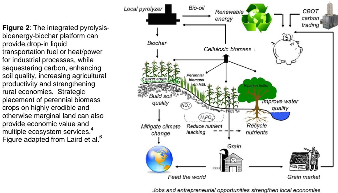
**Figure 2:** The integrated pyrolysis-bioenergy-biochar platform can provide drop-in liquid transportation fuel or heat/power for industrial processes, while sequestering carbon, enhancing soil quality, increasing agricultural productivity and strengthening rural economies. Strategic placement of perennial biomass crops on highly erodible and otherwise marginal land can also provide economic value and multiple ecosystem services.<sup>4</sup> Figure adapted from Laird et al.<sup>6</sup>
