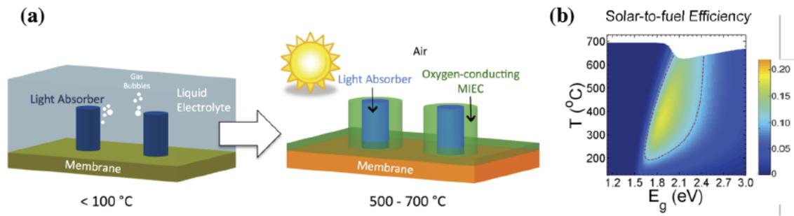
Figure 1: (a) Schematic comparison of the liquid-based PEC operating at room temperature versus the proposed solid-state (photo-anode) PEC operating at elevated temperature. (b) Simulated solar-to-fuel efficiency of the proposed PEC design. The white region indicates temperatures that are unreachable due to insufficient solar energy input. The dotted line indicates a 10% efficiency boundary.
