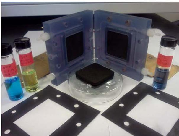
**Figure 1:** A disassembled laboratory-scale redox flow battery (RFB) cell for evaluation of new electrolyte chemistry and comparison with the all vanadium system. The cell uses flow-through porous electrodes and an ionomer membrane.
