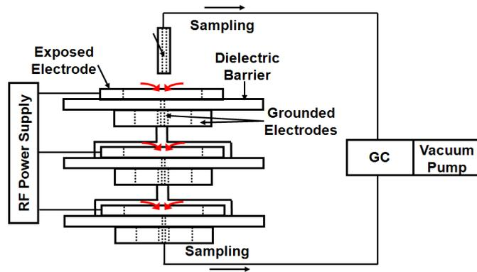
**Figure 7.** A typical schematic of a proposed multi-stage ASU.
