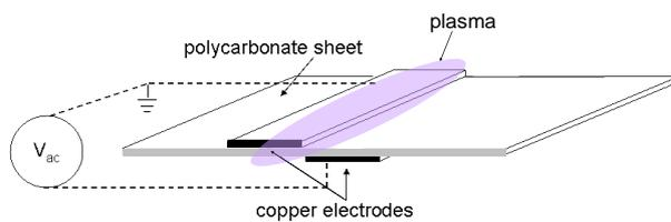
**Figure 1.** Schematic of a typical dielectric barrier discharge
