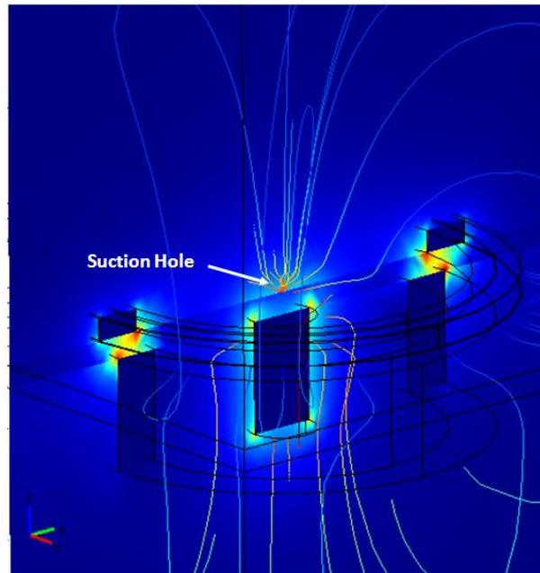
**Figure 5.** Electric field simulation in three dimensional view (Case III).
