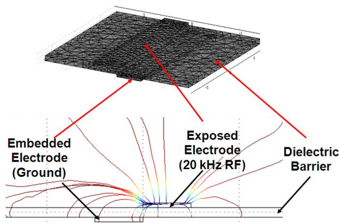
**Figure 3.** An electric field simulation conducted with a conventional DBD actuator.
