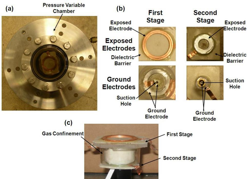
**Figure 8.** Two-stage PD-ASU built in a pressure variable chamber.
