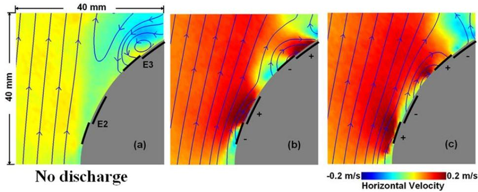
**Figure 2.** Phase Locked PIV images depicting negative ion ( $O_2^-$ ) attraction toward anode.
