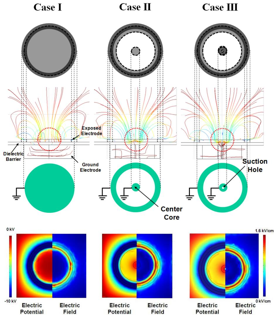
**Figure 4.** Electric field/potential simulated with various electrode designs.
