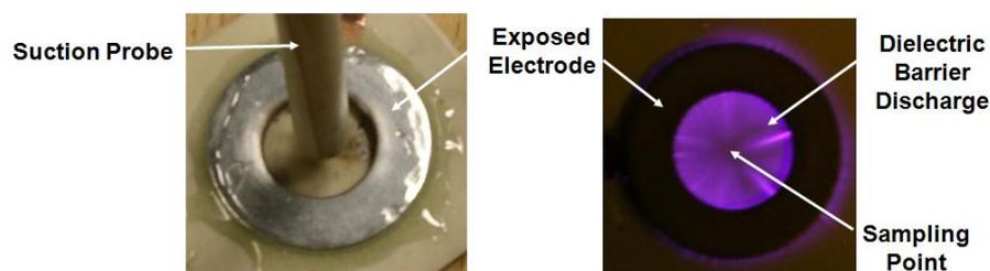
**Figure 6.** Photographs of a proposed ASU cell and the plasma discharge.
