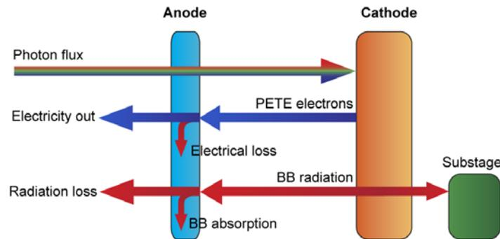
**Figure 2:** Energy flow for a tandem PETE/solar thermal cycle. Waste heat from the PETE device is used to power a conventional thermal engine, boosting the overall efficiency.
