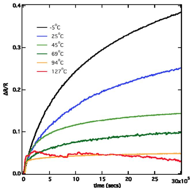
Fig. 11: Hydrogen uptake measured at different temperatures
