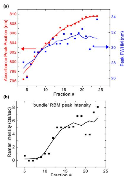
**Fig. 14:** Spectral properties of the SWNT optical transition near 800 nm. **(a)** Absorbance peak position and full-width at half-maximum tend to increase with increasing fraction number. The arrows indicate the absorbance peak position and FWHM, respectively, of the cholate-SWNT starting material, before DGC separation. **(b)** Peak intensity for the SWNT RBM feature at  $266\text{ cm}^{-1}$ , referred to as the “bundle peak,” following 785 nm excitation, with increasing fraction number.
