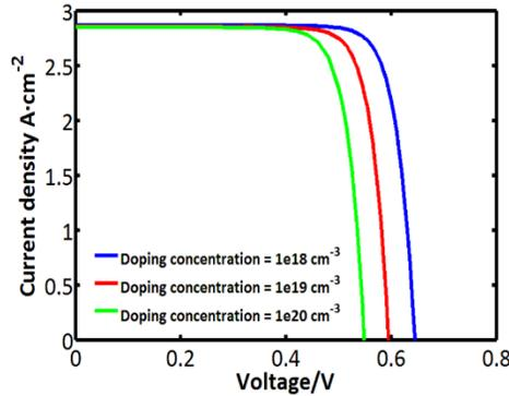
**Figure 5.** Simulation results of the InGaAs cell with different Window & BSF doping concentrations.
