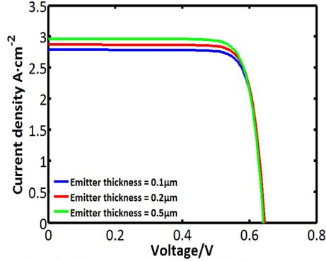
**Figure 6.** Simulation results of the InGaAs cell with different emitter thicknesses of 0.1  $\mu\text{m}$ , 0.2  $\mu\text{m}$ , 0.5  $\mu\text{m}$ .
