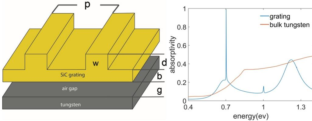
**Figure 2:** (a) (left) Schematic of the emitter design. (b) (right) Narrowband thermal emission peaking at 0.7eV.
