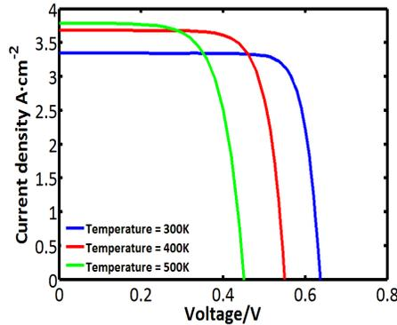
Figure 6. Simulation results of the optimized cell at different cell temperature of 300 K, 400 K, 500 K.
