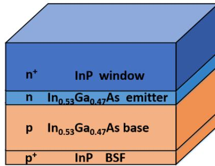
Figure 3. Schematic of the structure of the simulated  $\text{In}_{0.53}\text{Ga}_{0.47}\text{As}$  cell
