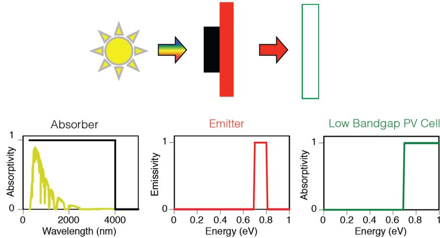
**Figure 1:** The concept of solar thermophotovoltaics. The black and red regions correspond to intermediate absorber and emitter, respectively. The green rectangle represents a narrow band gap cell.
