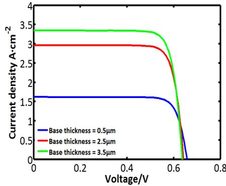
**Figure 7.** Simulation results of the InGaAs cell with different base thickness of 0.5  $\mu\text{m}$ , 2.5  $\mu\text{m}$ , 3.5  $\mu\text{m}$ .
