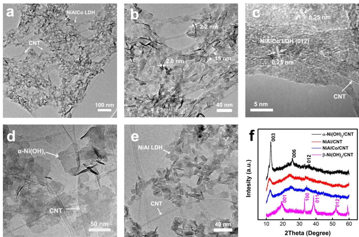
Figure 1. Characterization of size, morphology and structure of the hybrid materials. (a, b) TEM images of NiAlCo/CNT hybrid (c) HRTEM image of NiAlCo/CNT hybrid (d) TEM image of  $\alpha$ -Ni(OH)<sub>2</sub>/CNT hybrid (e) TEM image of NiAl/CNT hybrid (f) XRD spectra of NiAlCo/CNT hybrid (blue),  $\alpha$ -Ni(OH)<sub>2</sub>/CNT hybrid (black), NiAl/CNT hybrid (red) and  $\beta$ -Ni(OH)<sub>2</sub>/CNT hybrid (purple)
