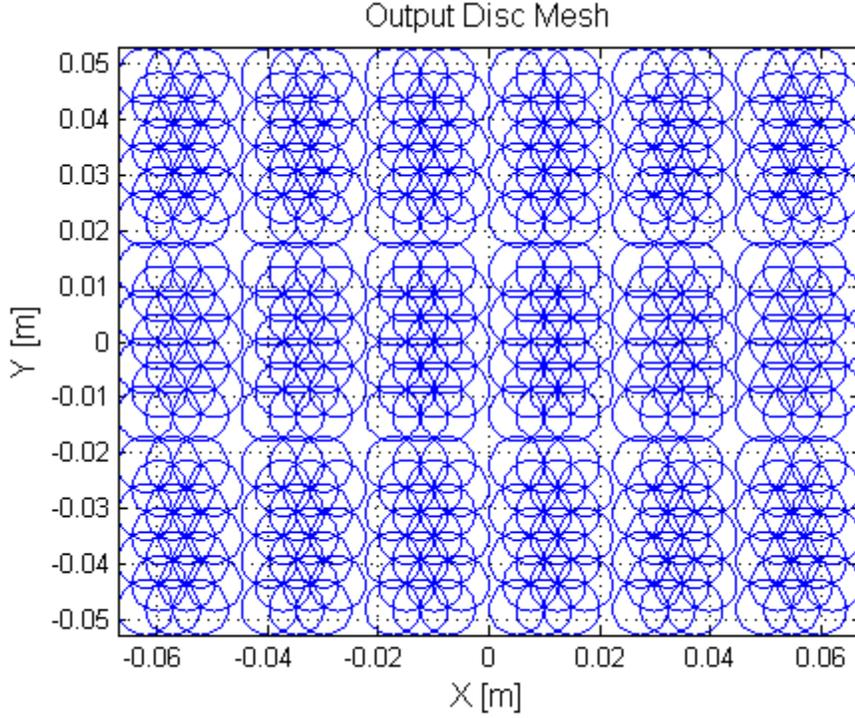
**Figure 4: Updated mesh of bulk superconductors based on meshing individual grains**
