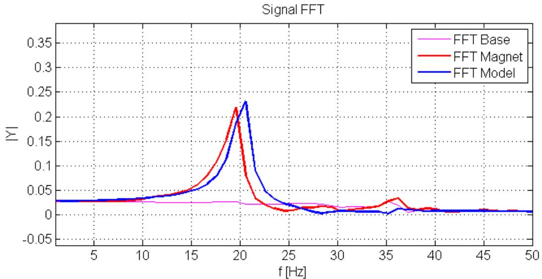
**Figure 6: FFT step response of lumped parameter model using grain mesh technique with additional viscous damping**
