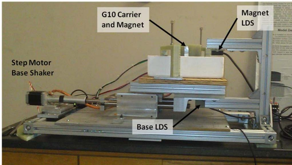
**Figure 1: Test setup for dynamic transverse model validation**
