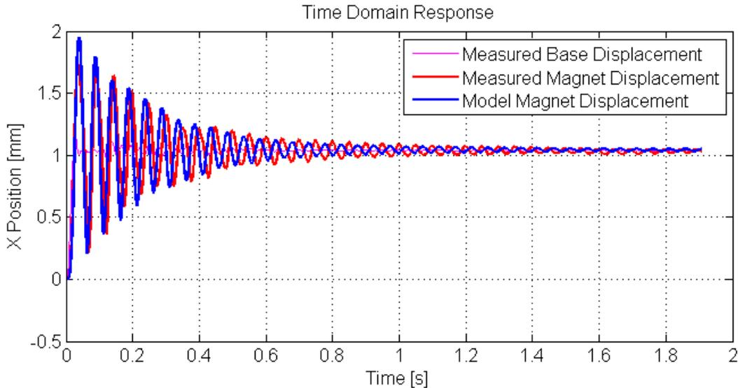
**Figure 5: Time domain step response of lumped parameter model using grain mesh with additional viscous damping**
