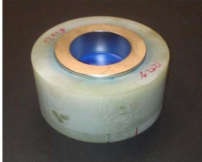
**Figure 3 Permanent magnet bonded in G10 carrier for dynamic test.**
