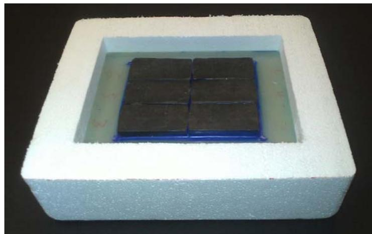
**Figure 2: Base of bulk YBCO superconductors for dynamic transverse test**
