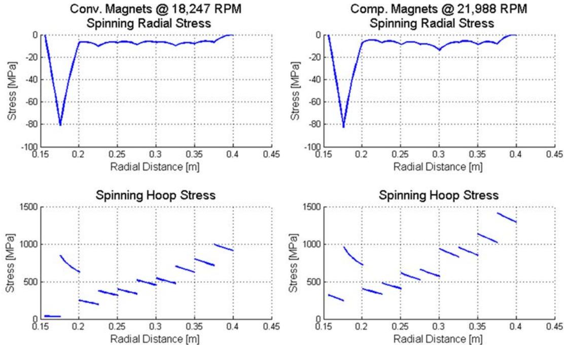
**Figure 9: Nested ring analysis results; Right: Flywheel with conventional permanent magnet segments on bore ID. Left: Flywheel with magnetically filled composite on bore ID**
