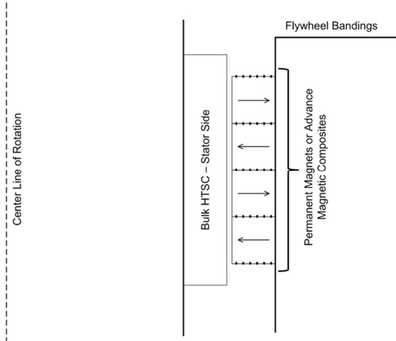
**Figure 7: Axissymmetric view of typical HTSC journal bearing design**
