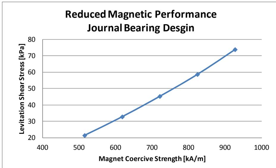
**Figure 8: Analysis using lumped parameter axisymmetric model for estimating reduction in journal bearing lifting capacity with reduced magnetic performance**
