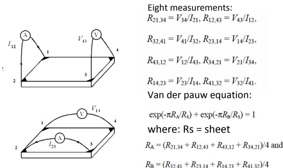
Figure 2. Schematics and details of the Van der paum measurement that will be used to determine the sheet resistance of ZnO based TOC films.
