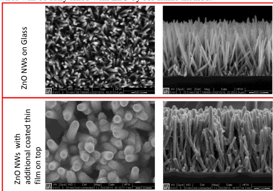
Figure 1. Scanning electron microscope images of (top) ZnO nanowire arrays grown on glass substrates; (bottom) ZnO nanowire arrays that are further coated with ZnO shells by the sol-flame method.
