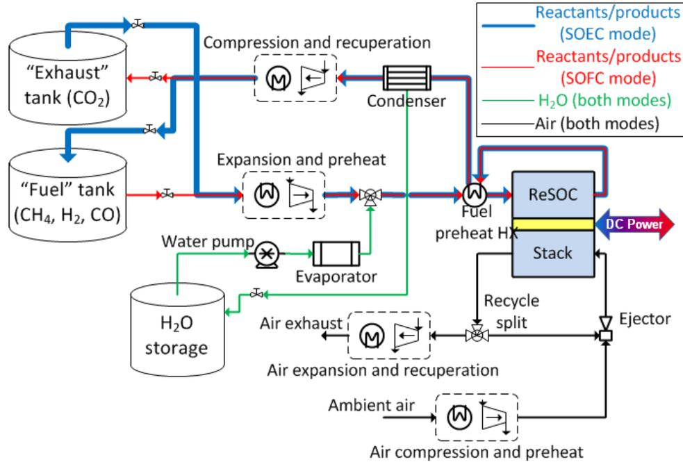
**Figure 24. Energy storage system schematic**
