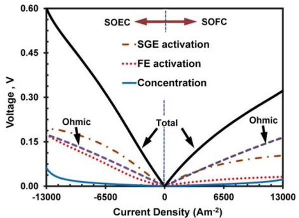
**Figure 20. Break down of polarisation losses versus cell current density at  $750^\circ\text{C}$**
