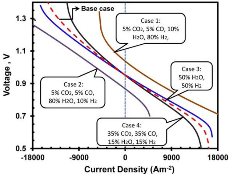
**Figure 21. V-j characteristic curve at 850°C with different feedstock gas composition**
