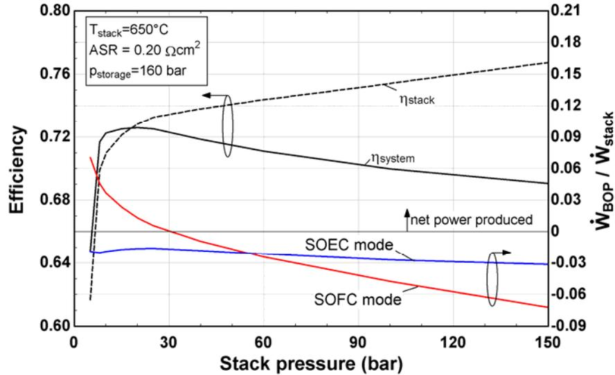
**Figure 27. Stack and system efficiency (left) and BOP power relative to stack power (right) vs. stack pressure [22]**
