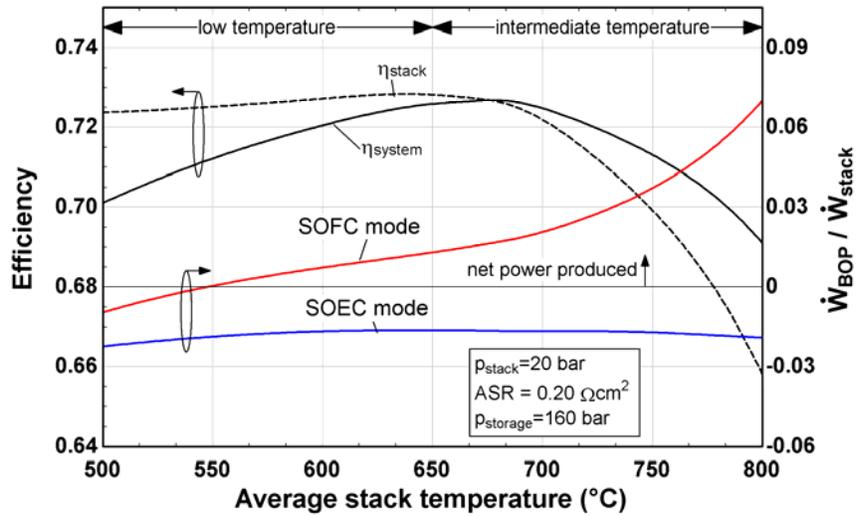
**Figure 29. Stack and system efficiency (left) and BOP power relative to stack power (right) vs. stack temperature [22]**
