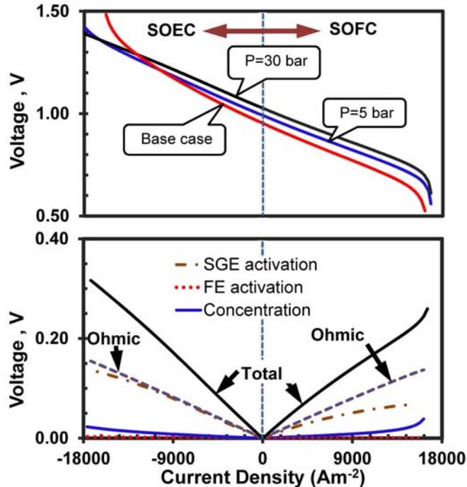
**Figure 22. V-J characteristic curve and break-down of the cell polarizations for pressurized operation**
