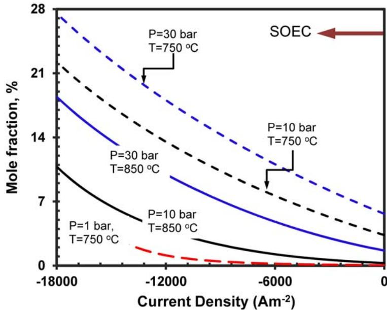
Figure 23. Outlet mole fraction of  $\text{CH}_4$  at different pressures and temperatures
