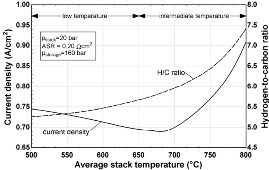
Figure 28. Current density and hydrogen-to-carbon ratio vs. stack temperature [22]
