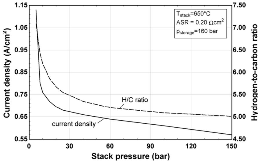
Figure 26. Current density and hydrogen-to-carbon ratio vs. stack pressure [22]
