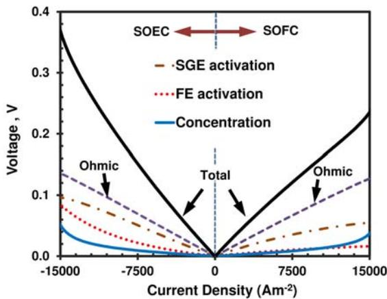
**Figure 19. Break down of polarisation losses versus cell current density at  $850^\circ\text{C}$**
