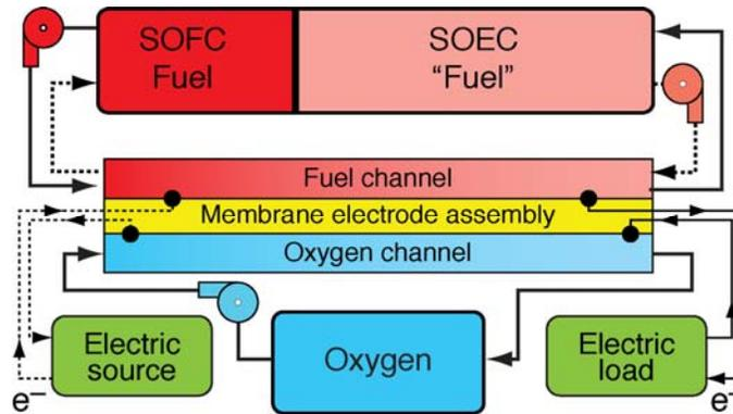
**Figure 1. Simplified process flow diagram for the SOFB concept. Discharging is shown with solid lines and charging with dashed lines.**
