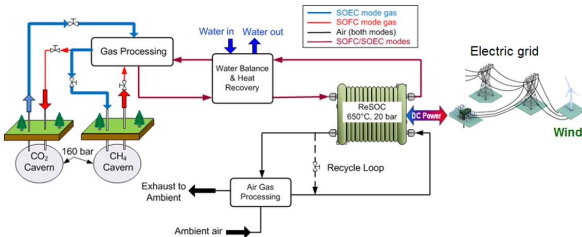
**Figure 30. System concept for large-scale GWh energy storage using SOFB technology**
