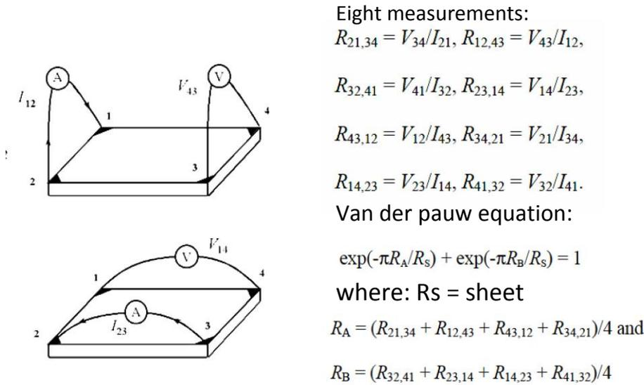
Figure 2. Schematics and details of the Van der pauw measurement that will be used to determine the sheet resistance of ZnO based TOC films.
