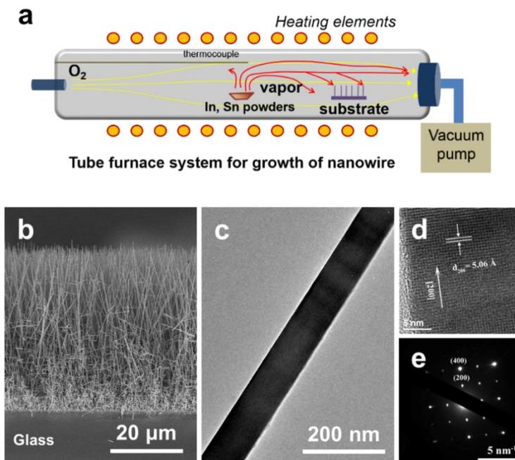
Figure 3. a) Schematic illustration of vapor transport method for synthesis of ITO nanowire arrays. b) Scanning electron microscopy image of ITO nanowire arrays grown on the ITO/Glass substrate. c) Transmission electron microscopy image, d) High-resolution transmission electron microscopy image and e) selected-area electron diffraction (SAED) pattern of single ITO nanowire.
