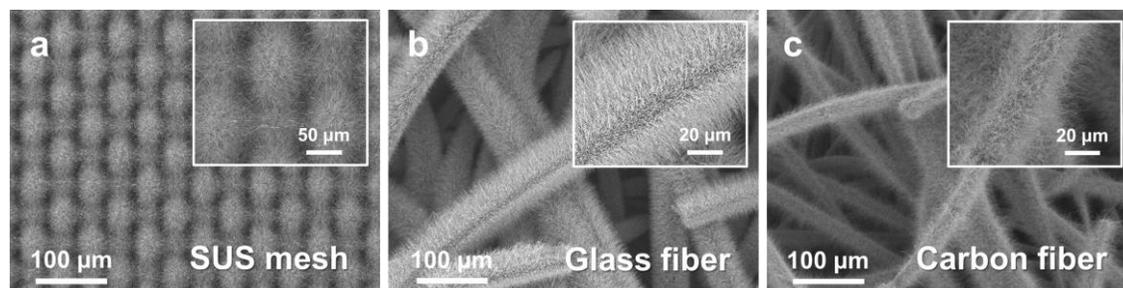
Figure 4. Scanning electron microscopy images of ITO nanowire arrays grown on a) stainless steel meshes, b) glass fibers and c) carbon fibers.
