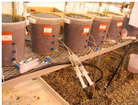
Figure 5. Mesocosm experimental system for methane and carbon dioxide production in rice paddy soils.
