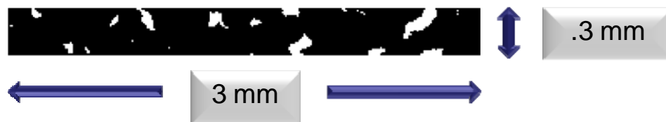
Figure 9: Example size of a discrete thin section element.
