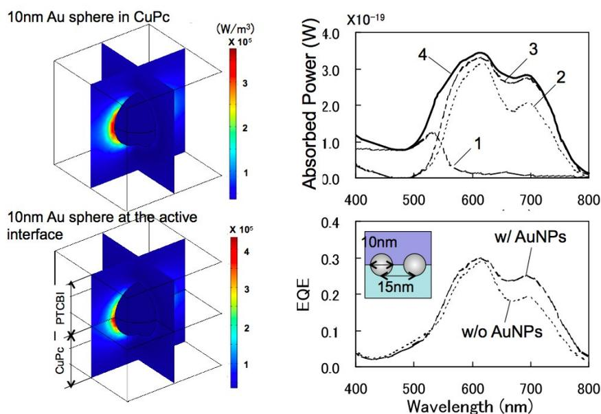
**Figure 1:** The presence of a 10nm-diameter gold nanoparticle in an organic matrix leads to increased optical absorption (top) and increased device performance (bottom) according to finite-element simulations.
