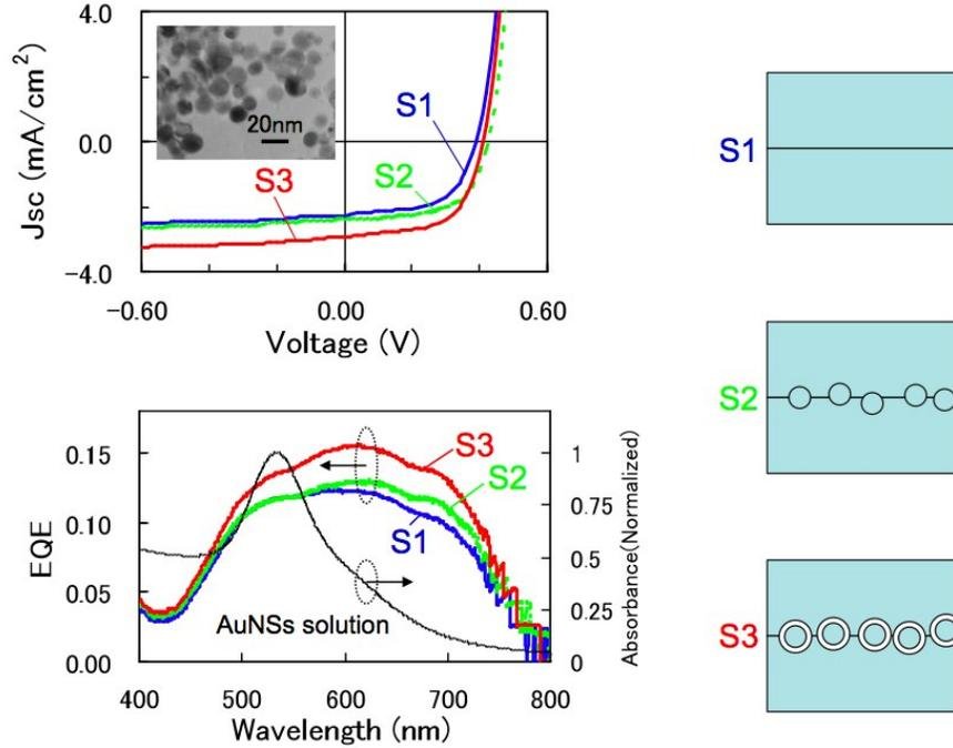
**Figure 2:** (Top) Increase in photocurrent for a bilayer cell when metal nanoparticles are included at the interface between the donor and acceptor of a simple bilayer organic solar cell. S1 is a control device without metal nanoparticles, S2 is a device with metal nanoparticles coated with an alkanethiol and S3 is a device in which a thin wide-bandgap coating was used to further electrically isolate the nanoparticles from the organic matrix. (Bottom) Increase in external quantum efficiency.
