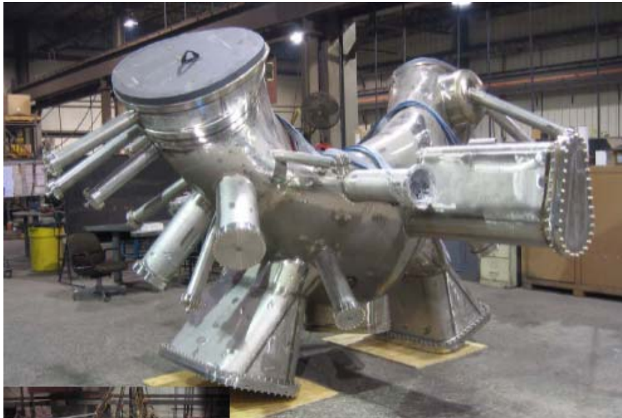
Segment #1 of 3 Sealed for Pump-down
