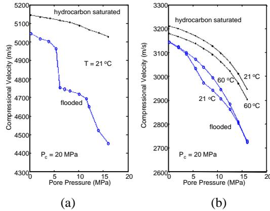
Figure 7. The velocity of compressional waves in CO<sub>2</sub>-saturated sandstone is significantly less than oil-saturated sandstone. (a) measured velocities (Nur and Wang, 1989); (b) modeled velocities calculated from the Gassmann fluid substitution model and a trial pressure dependence. Shear velocities do not change significantly due to saturation changes.
