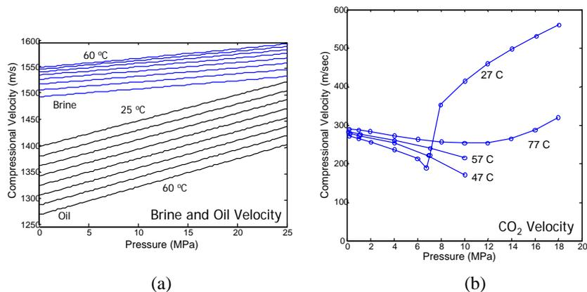
Figure 6. The velocities of compressional waves in the component fluids are important for estimating the velocity of a CO<sub>2</sub>-saturated mixture: (a) velocity in typical brines and oils; (b) velocity in CO<sub>2</sub><sup>2</sup>.
