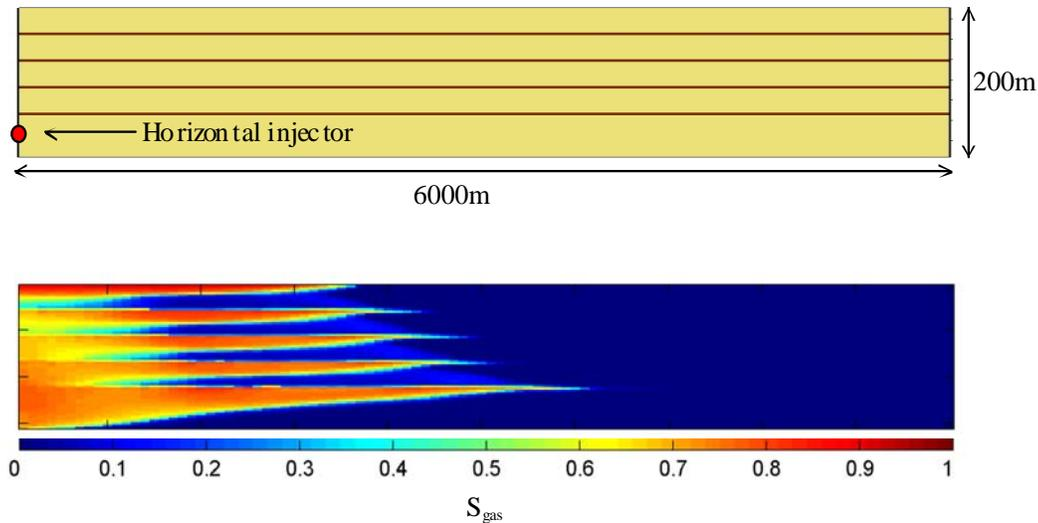
Figure 1. Simplified model of the Utsira formation (top). Low permeability shales are darkly shaded and high perm sands are light. Prediction (lower) of CO<sub>2</sub> distribution after 2 years of injection.
