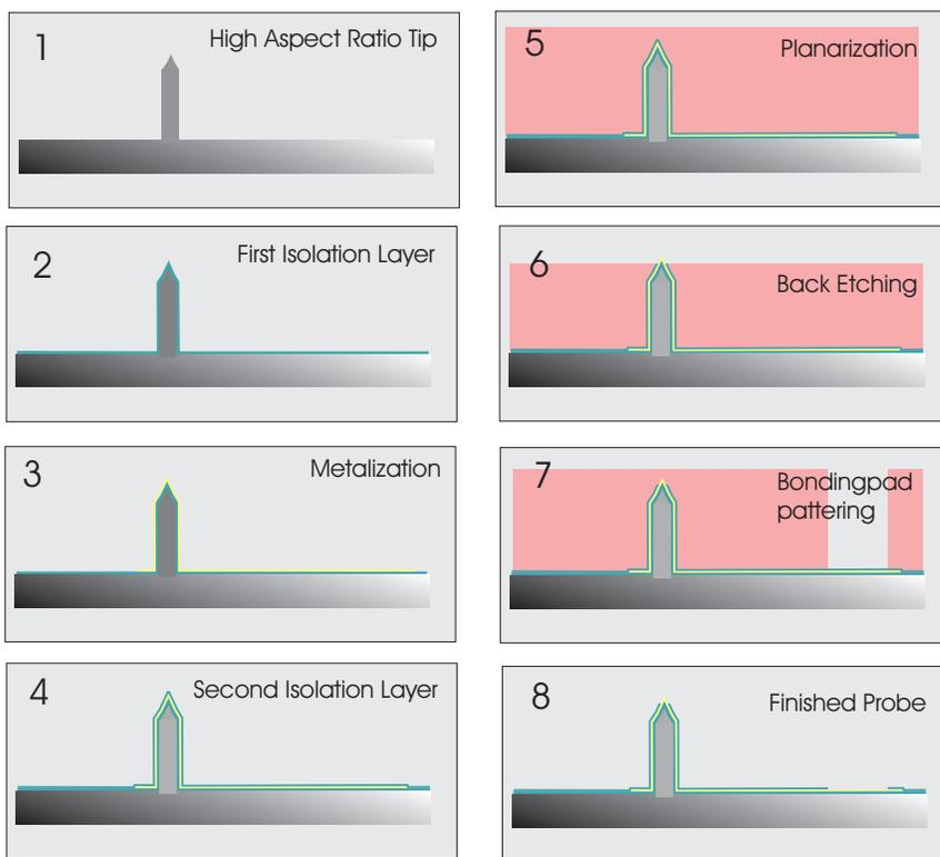
Figure 1. Fabrication of the pencil probes: (1) Starting with HARS tips, (2) Deposition of LPCVD Silicon nitride as an Isolation layer, (3) Deposition and patterning of a metal layer, (4) Deposition of the PECVD Silicon nitride as an passivation layer, (5) Planarization using thick photo resist, (6) Etch-back of resist and silicon nitride layer to expose the buried metal layer, (7&8) patterning and etching of the bonding pads.
