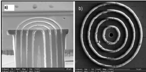
Figure 4: A  $40\mu\text{m}$ -diameter ETWI consisting of four  $2\mu\text{m}$ -thick poly-silicon layers and four  $1\mu\text{m}$ -thick thermal silicon-oxide layers (a) SEM image of the cross section (b) SEM image of the top view (poly-silicon and silicon appears as dark, silicon-oxide appears as bright).
