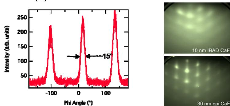
**Figure 1.** RHEED images and (220) phi scan for an IBAD  $\text{CaF}_2$  film with a 30 nm homoepitaxial layer.
