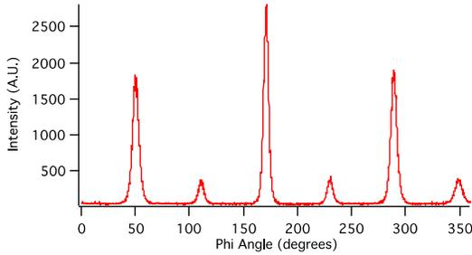
**Figure 7.** XRD Phi scan of Ge (220)
