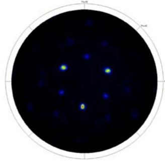
**Figure 8.** XRD Pole Figure of Ge film
