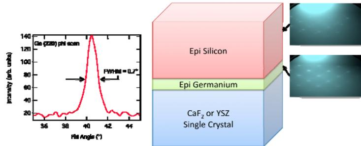
**Figure 2.** An illustration of the architecture used for the proof of principle experiments used to determine whether Si can be deposited on  $\text{CaF}_2$ . The XRD phi-scan on the left shows the epitaxial nature of the Ge layer deposited on  $\text{CaF}_2$ .
