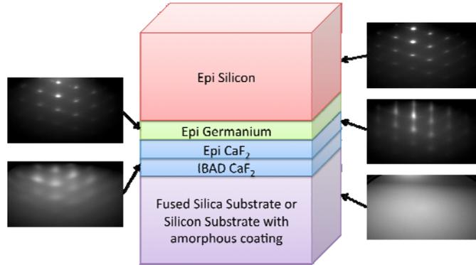
**Figure 3.** An illustration of the architecture used for the IBAD  $\text{CaF}_2$ -templated polycrystalline Si structure. The accompanying RHEED images were taken at the conclusion of each layer's growth.
