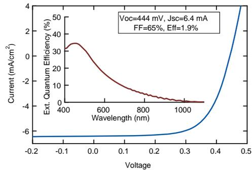
**Figure 10.** IV and EQE of our 1<sup>st</sup> solar cell
