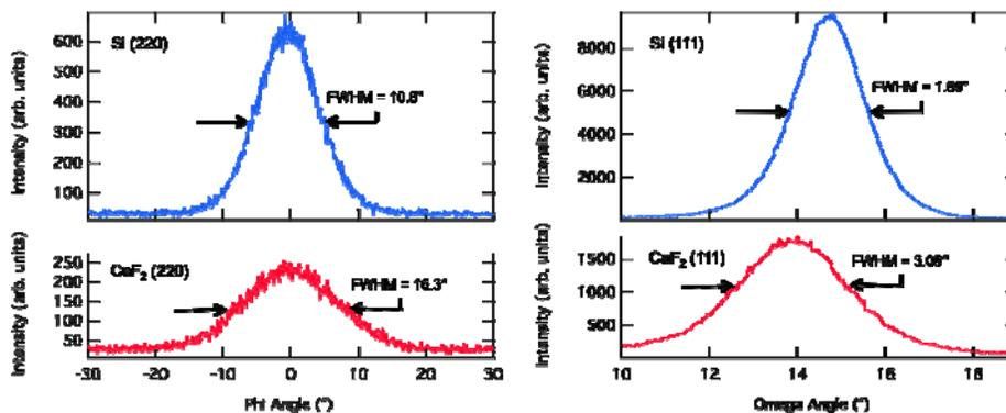
**Figure 4.** The XRD spectra of a film with the architecture illustrated in Figure 4. On the left are phi-scans of the  $\text{CaF}_2$  (lower left) and Si (upper left) (220) peaks with FWHM of  $16.3^\circ$  and  $10.8^\circ$ , respectively. On the right-hand side are the omega (out-of-plane) scans for the (111) peaks of the two layers.
