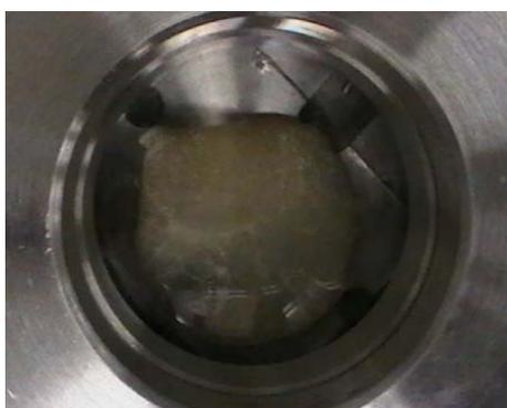
**Figure 9:** Membrane in a high pressure cell for SC-CO<sub>2</sub> treatment.
