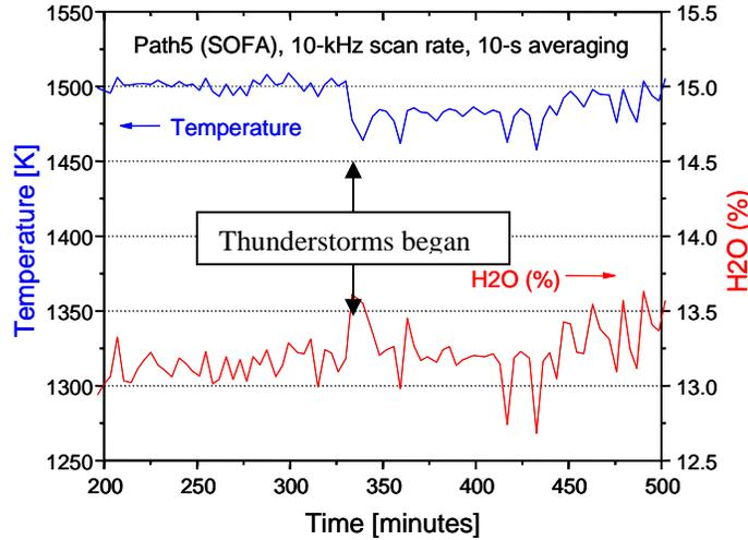
**Figure 4:** Gas temperature and water vapor concentration in the coal combustor of a 280MW power plant at full load, and illustrates the influence of weather on the combustion gases.
