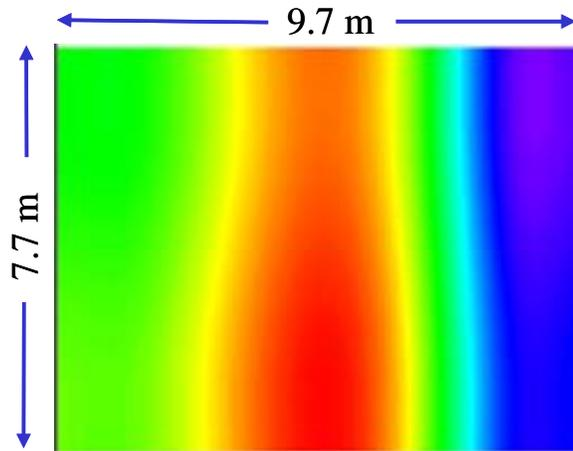
**Figure 5:** Coarse tomographic reconstruction of the temperature field (max 1528K (red) and minimum 1425K (blue)) at a location 10 m above the 280MW combustor at the position for injection of secondary over-fire air.
