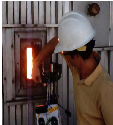
Figure 3: Adjustment of the optical collection near an access port used for preliminary measurements. Note the bright emission from the hot particulate coal and soot is evident. Successful wavelength-tuned sensor measurements are made even though this particulate limits the optical transmission to less than 1%.
