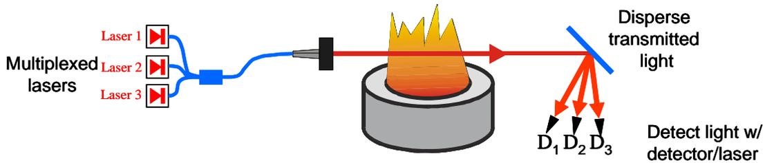
**Figure 2:** Wavelength-multiplexed absorption concept for **smart optical sensors**.
