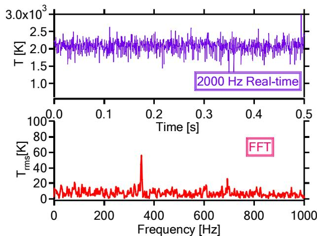
**Figure 8:** Real-time gas temperature measurements at 2kHz (top panel). Power spectrum of temperature data captures frequency of flame instability (lower panel); flame instabilities limit the practical implementation of low NO<sub>x</sub> industrial burners.
