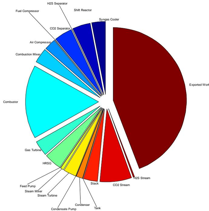
**Figure 1:** Exergy analysis of an IGCC plant with CO<sub>2</sub> separation. The largest fraction of fuel exergy is exported as work, while the largest exergy destruction takes place in the gas turbine's combustor.
