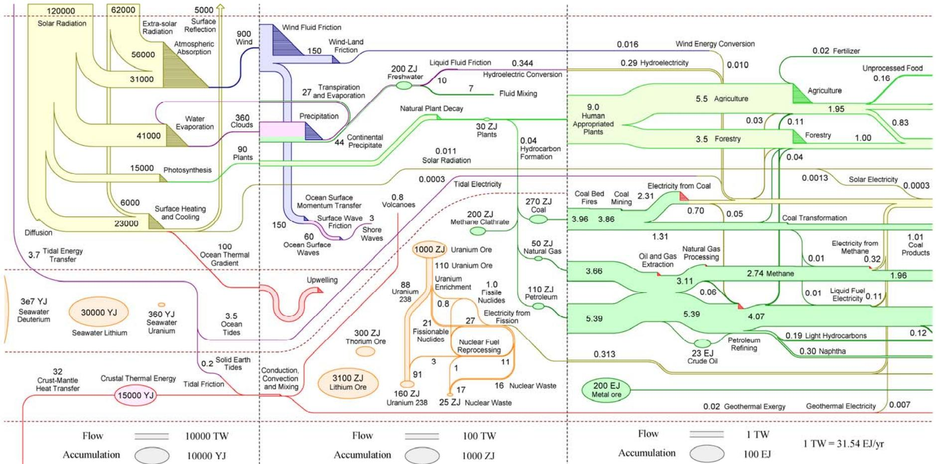
**Figure 2a** : Global exergy flow, accumulation and destruction (continued in Figure 2b). Brown dotted lines represent the boundaries of the system of interest: that under anthropogenic influence between the stratosphere-mesosphere and crust-mantle interfaces. Black dotted lines designate scale changes (see legend at bottom, this page). Exergy flow is generally from left to right. Color codes are provided in the continuation of this figure on the next page.
