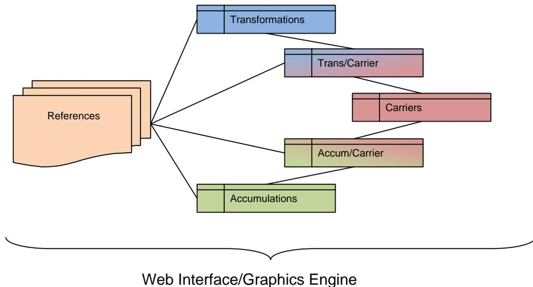
**Figure 3:** The database is structured so that a query language can process real interconnections between energy carriers, transformations and resources. In this representation, the complex structure of the reference table has been collapsed for readability.
