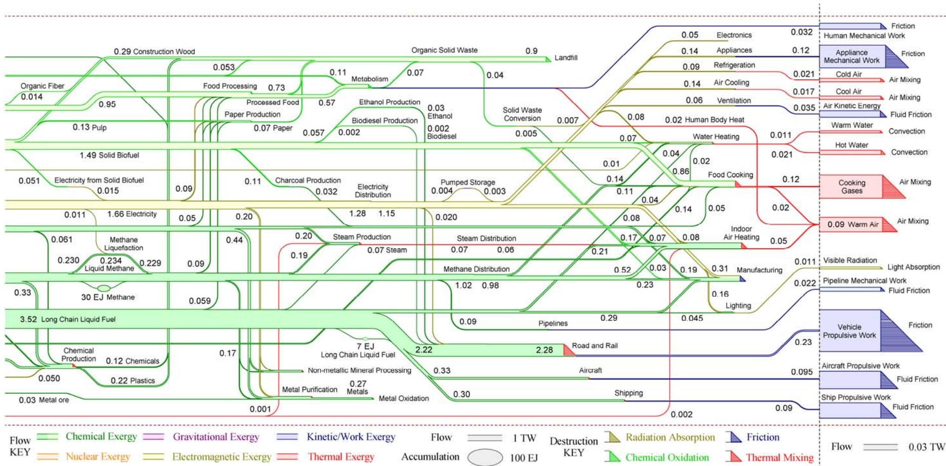
**Figure 2b** : Global exergy flow, accumulation and destruction (continued from Figure 2a). Brown dotted lines represent the boundaries of the system of interest: that under anthropogenic influence between the stratosphere-mesosphere and crust-mantle interfaces. Black dotted lines designate scale changes (see legend at bottom, this page). Exergy flow is generally from left to right.
