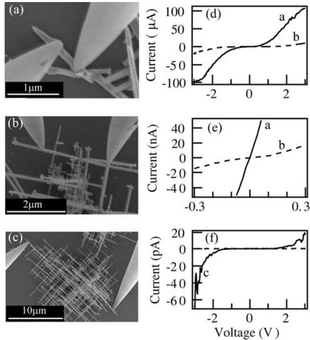
**Figure 5** (a) to (c) are SEM images of hyperbranched NW networks contacted by two tungsten probes. (d) is I-V data with curve a and b corresponding to the cases in (a) and (b), respectively. (e) is the low bias region of (d). The solid line in (f) is the I-V data for (c) and the dashed line is the I-V data through the substrate.
