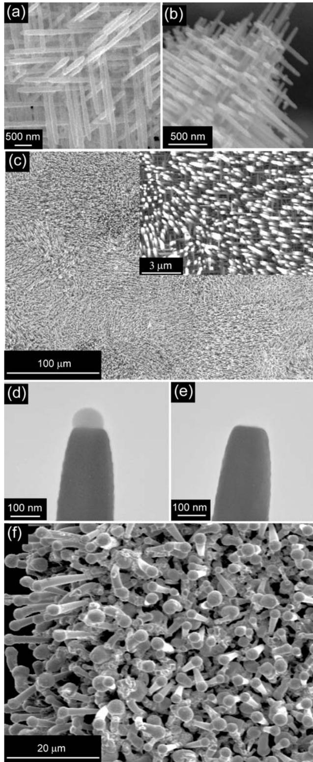
**Figure 3.** (a) (b) SEM images of PbSe NWs using Indium, Gallium as catalyst, growth for 60 min; (c) SEM image of PbSe NWs using Bismuth as catalyst, growth for 120 min, inset is a zoomed in picture; (d) (e) TEM image of PbSe NWs with and without Bi particles; (f) SEM image of PbSe NWs with Bi particles at the end.
