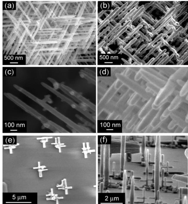
**Figure 4** (a) (b) SEM images of PbSe NWs with different growth temperature: 650°C and 700 °C, respectively, (c) (d) SEM images of PbSe NWs with different Indium temperature: 350°C and 400 °C respectively, (e) and (f) top-view and cross-section SEM images of epitaxial growth of PbSe NWs on NaCl <001> substrate.
