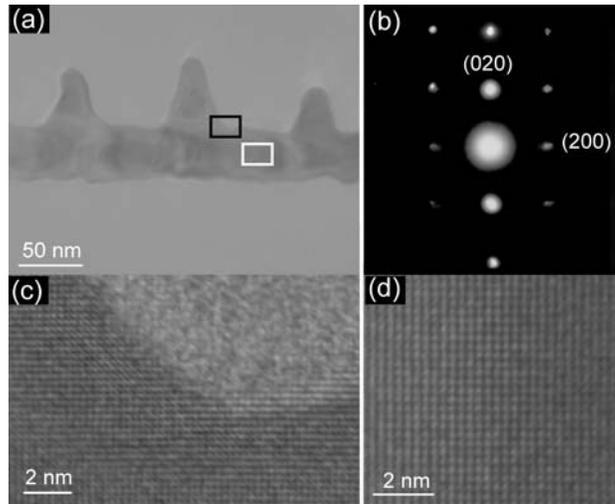
**Figure 2.** (a) TEM image of a branched PbSe NW. (b) and (c) SAD pattern and HRTEM image of the PbSe NW obtained at the branching interface (black rectangular in (a)), respectively. (d) HRTEM image of the main PbSe NW (white rectangular in (b)).
