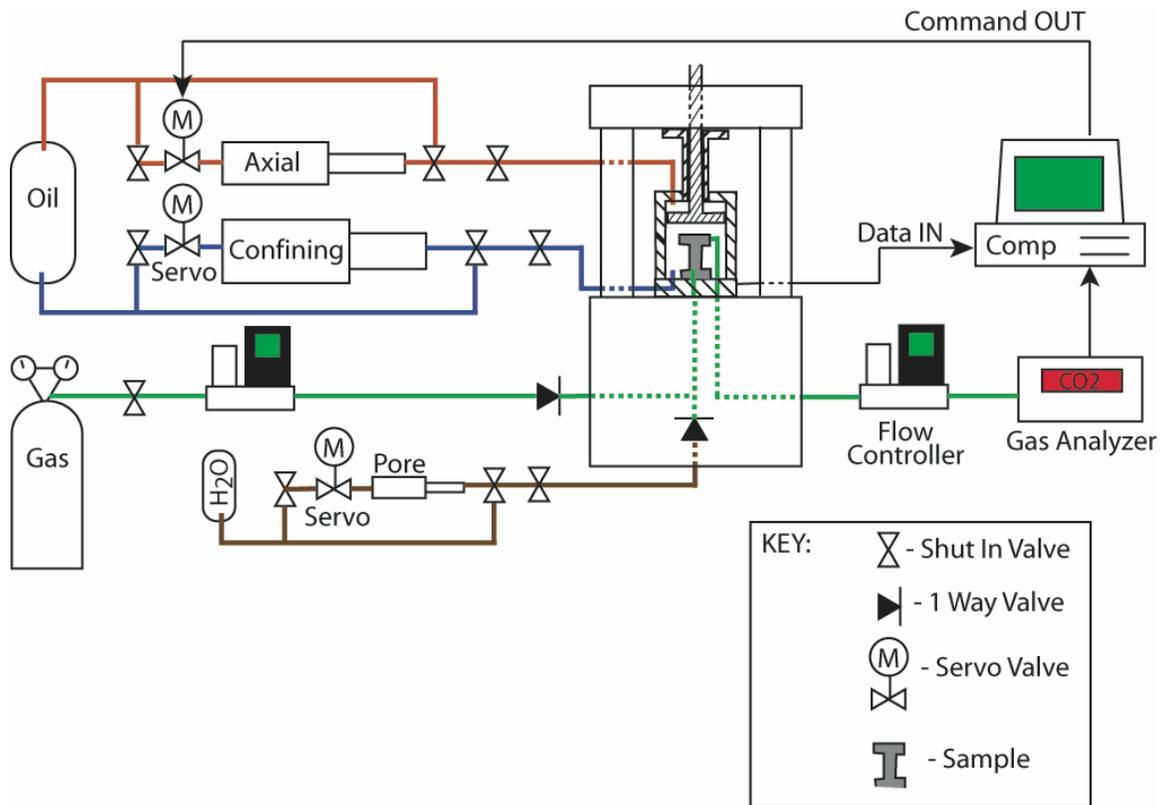
**Figure 1.5:** Schematic view of the completed laboratory apparatus. Items connected by the green hydraulic lines (Gas canister, flow controllers, analyzer) represent the new equipment added to the system.
