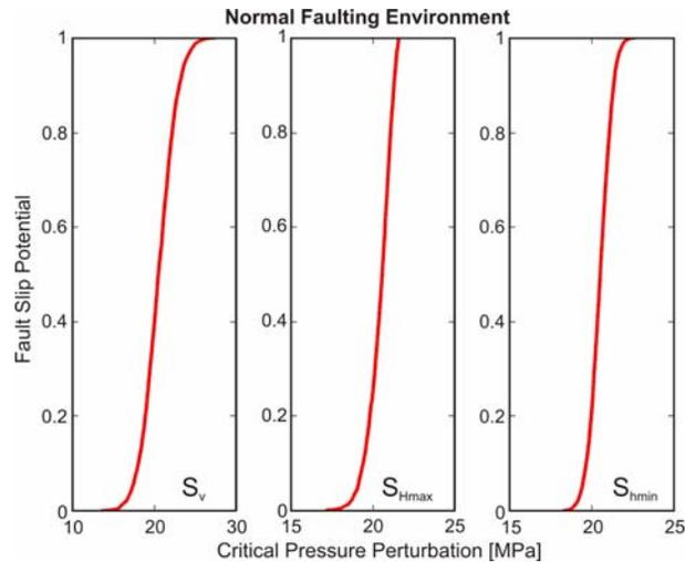
**Figure 1.2:** Fault slip potential probability for Normal Fault environment, as function of each of the components of the stress tensor, varying  $S_1$  (maintaining  $S_2$  and  $S_3$  fixed) (left); varying  $S_2$  (maintaining  $S_1$  and  $S_3$  fixed) (center) and varying  $S_3$  (maintaining  $S_1$  and  $S_2$  fixed) (right).
