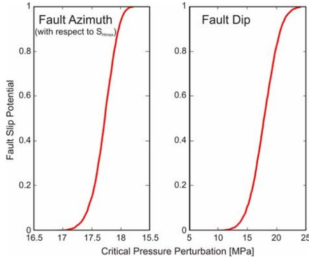
**Figure 1.4** Fault slip potential probability as function of variation in the fault azimuth (left) and in the fault dip angle (right). The mean value of the stress tensor was used to analyze these scenarios.
