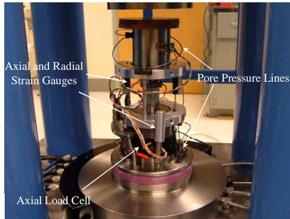
**Figure 1.6:** Photograph showing modified coreholder assembly, including new pore pressure lines for gas permeability measurements. A coal sample core can be seen in the center of the coreholder assembly, jacketed in Teflon heatshrink tubing.
