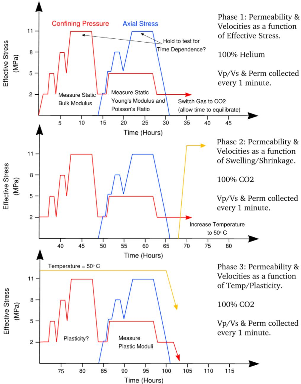
**Figure 1.7:** Schematic diagram describing the experimental plan for the Powder River Basin coal samples. Both powdered and intact coal samples will be tested following this general procedure. See the text for details.
