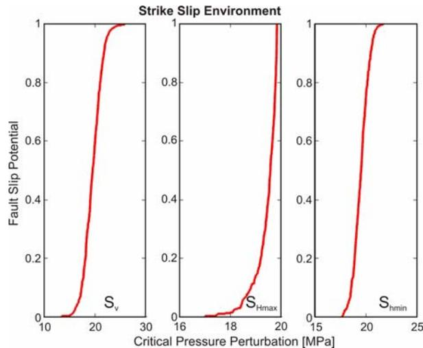
**Figure 1.3:** Fault slip potential probability for Strike-Slip environment, as function of each of the components of the stress tensor, varying  $S_1$  (maintaining  $S_2$  and  $S_3$  fixed) (left); varying  $S_2$  (maintaining  $S_1$  and  $S_3$  fixed) (center) and varying  $S_3$  (maintaining  $S_1$  and  $S_2$  fixed) (right).
