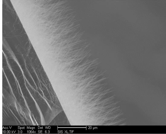
**Figure 1:** A SEM of SiNWs grown off a Si substrate.
