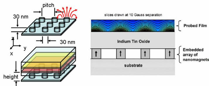
**Figure 3:** Concept of electron spin resonance imaging using arrays of nanomagnets to create very steep gradients in magnetic field that can be used to “slice” a layer under investigation into nm-thick regions.
