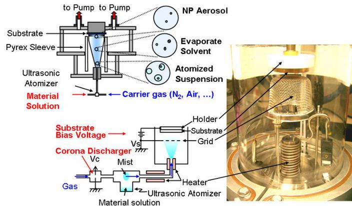
**Figure 1:** Schematic diagram and photograph of the optimized aerosol deposition tool that was recently developed in our lab.
