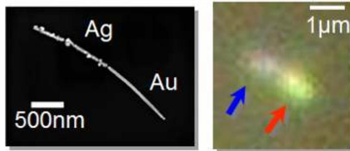
**Figure 7:** (a) Scanning electron microscopy (SEM) image of a hybrid Ag/Au nanowire generated by electroplating of Ag and Au into a porous polycarbonate membrane (b) Dark-field optical microscopy image of the same wire. The blue and red arrows indicate the location of the Ag and Au sections of the wire.
