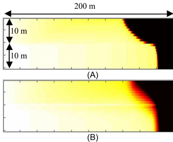
**Figure 1. (A) Displacement front without accounting for capillarity:** Illustrates the introduction of capillary effects during water flooding in a two-dimensional two-layer oil reservoir. The top layer is less permeable than the bottom. White shading represents water and dark shading represents oil.
