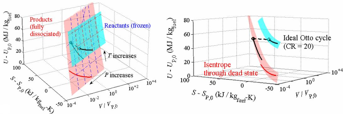
**Figure 1:** Internal energy/entropy/volume thermodynamic surfaces for stoichiometric propane/air. The ideal, reactive Otto cycle is depicted by the black lines while an isentrope with products expanded to the thermal dead state ( $T_0 = 300$  K,  $P_0 = 1$  atm) is shown in red.
