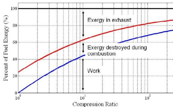
**Figure 1:** Combustion of uncompressed, unheated reactants destroys 25% of the work potential of the fuel. Increasing the internal energy of the reactants before combustion by about 40%—through compression, heating, or any combination of the two—can cut this loss in half, resulting in the potential for a significant increase in
