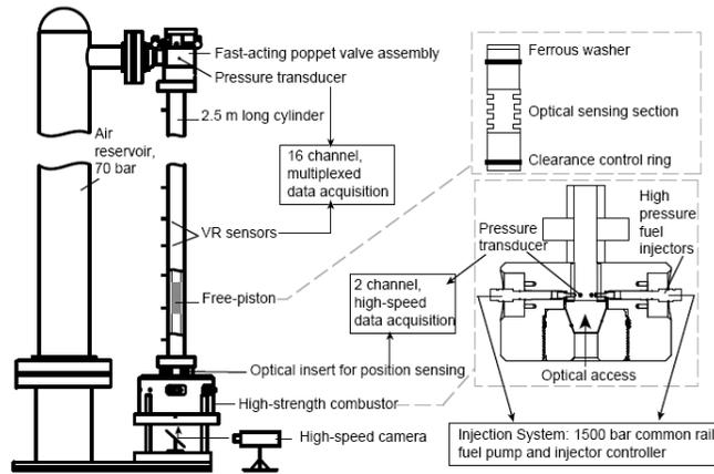
The key research challenge remaining for an extreme compression engine is design and execution of an optimal combustion strategy.
