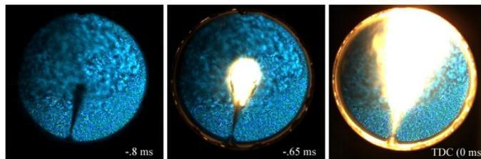
The images are obtained via a combination of schlieren and direct photography that permits simultaneous imaging of gas-phase density gradients, spray extinction, and combustion luminosity on a single camera.
