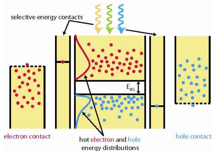
**Figure 1:** Band diagram of a hot carrier solar cell. Energy distributions of hot electron and hole populations created by photon absorption are shown together with selective energy contacts and cell electrodes.
