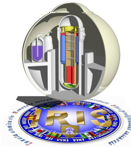
International Reactor Innovative and Secure (IRIS) 335MWe
