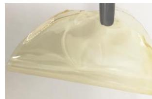
**Figure 2.** Synthesis of CANAL-polyimides (PIs) and CANAL-Tröger's base (TB) polymers. Photo shows the flexibility of formed polymer membrane.
