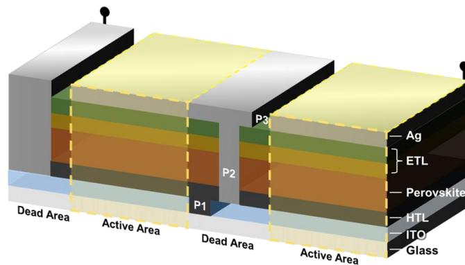
**Figure 7:** Layer cross section of perovskite module architecture showing scribing marks used to isolate and then connect individual subcells.
