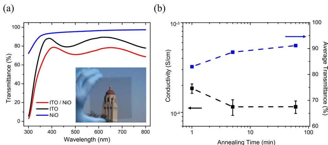
**Figure 2:** (a) Visible range transmittance of large area sprayed NiO films. (b) Conductivity and average transmittance of NiO films as a function of post-annealing time at 300 °C.
