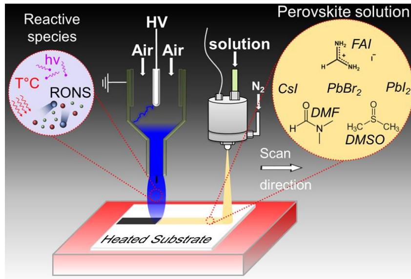
**Figure 5:** Schematic illustrating rapid spray plasma processing (RSPP) of perovskite double cation  $\text{Cs}_{.17}\text{Fa}_{.83}\text{Pb}(\text{I}_{.83}\text{Br}_{.17})_3$  absorber films.
