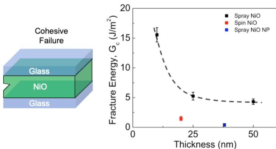
**Figure 4:** (a) Double cantilever beam fracture energy test structure. (b) Measured fracture energy of NiO films produced by aqueous spray coating (black) vs spin coating (red) and sprayed NiO nanoparticles (blue).
