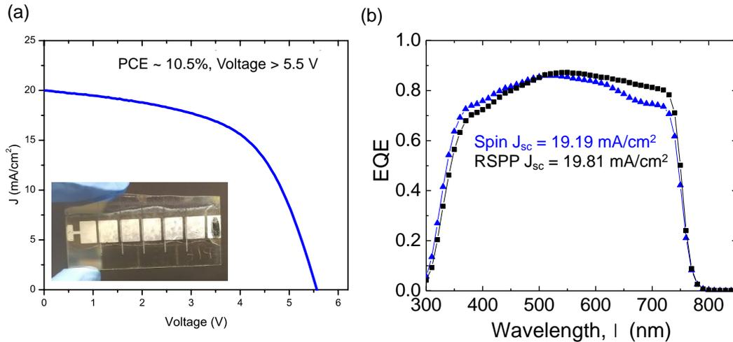
**Figure 8:** (a) Current-voltage characteristics of spray-plasma fabricated perovskite module formed by series-integration of 6 individual subcells. (b) External quantum efficiency (EQE) of perovskite subcells formed by rapid spray plasma processing (RSPP).
