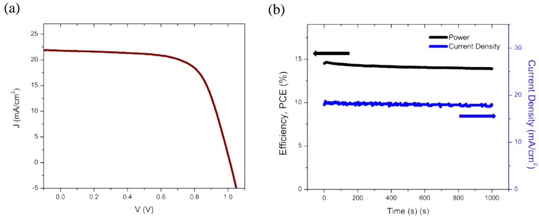
**Figure 6:** (a) Current-voltage characteristic of plasma-processed perovskite solar cell and maximum power point tracking stability under full illumination (b).
