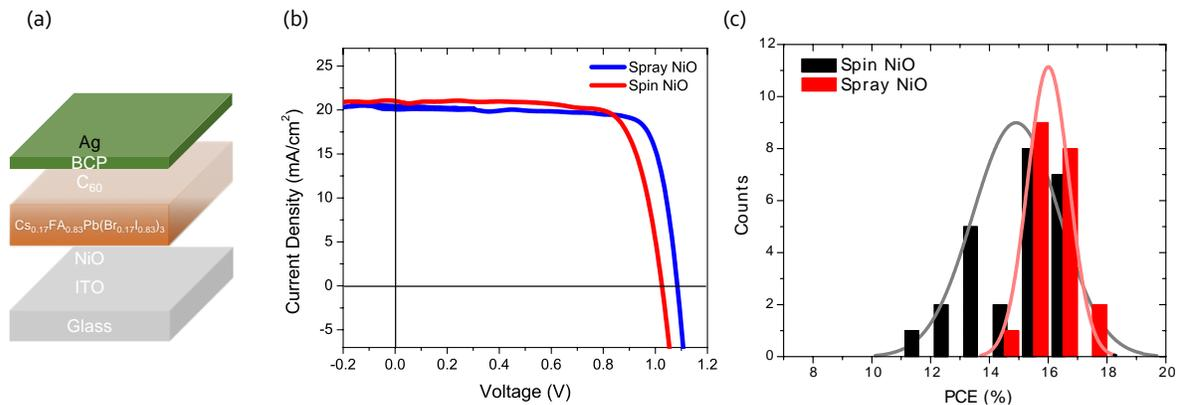
**Figure 3:** (a) Layer architecture of perovskite cells and modules reported here. (b) Comparison of current-voltage characteristics of perovskite cells with spin coated and spray coated NiO films. (c) Distributions of device efficiencies for perovskite cells incorporating spin (red) coated and spray coated (black) NiO hole transport layers.
