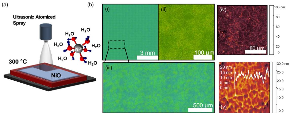
**Figure 1:** (a) Ultrasonic spray deposition of NiO transport layers. (b) Micrographs (i-iii) of NiO films with height maps measured by stylus profilometry (iv) and AFM (v).
