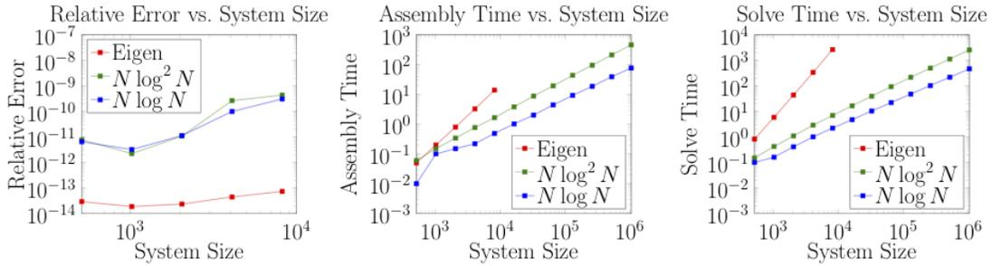
Figure 6: Performance and accuracy of fast direct solver.
