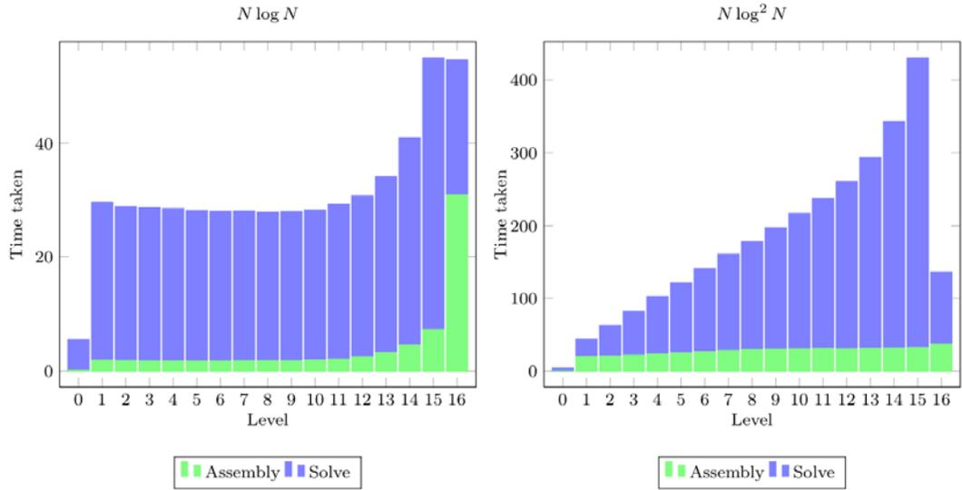
Figure 7: Time taken at each level in the hierarchy by the two fast algorithms.
