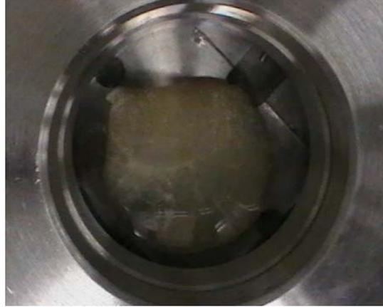
**Figure 9:** PAMAM dendrimer containing PEGDMA/TMPTMA membrane under sc-CO<sub>2</sub>.
