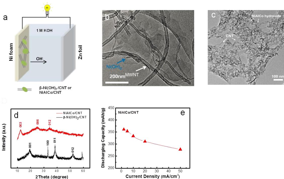
**Figure 1:** Rechargeable Ni/Zn batteries based on inorganic-CNT hybrid electrode materials. (a) A schematic showing the battery configuration, (b) SEM image of  $\beta$ -Ni(OH)<sub>2</sub>/CNT, (c) SEM image of NiAlCo/CNT. (d) XRD of  $\beta$ -Ni(OH)<sub>2</sub>/CNT and NiAlCo/CNT, (e) dependence of specific capacity on discharge current density for NiAlCo/CNT tested in a three electrode system.
