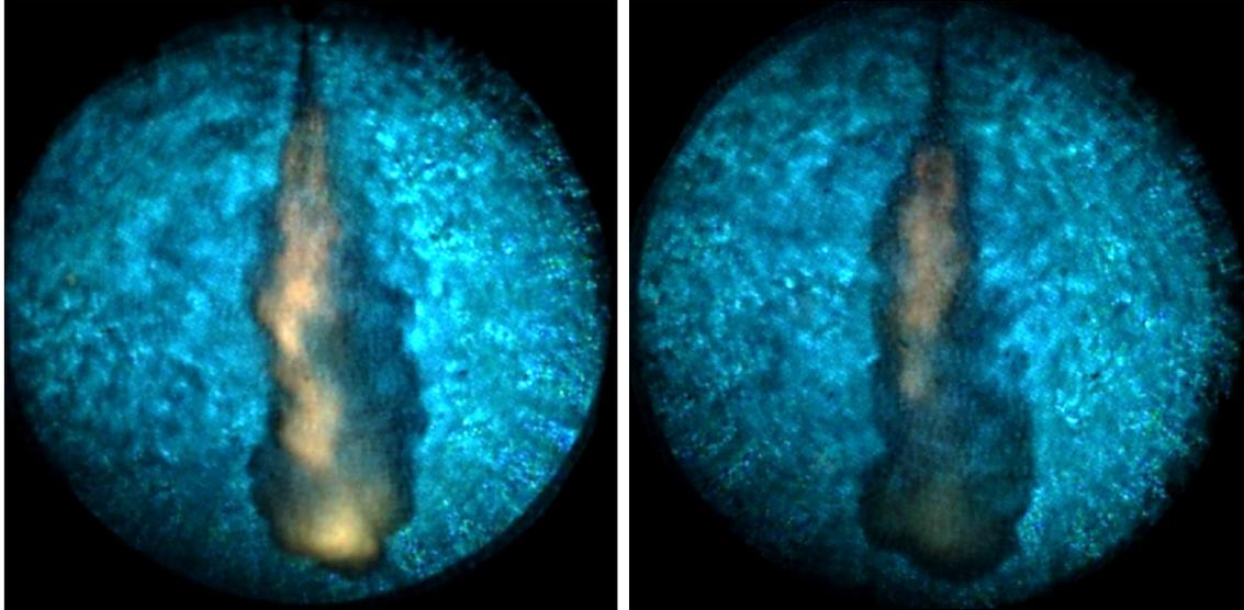
**Figure 2:** Comparison between neat methanol (left) and a 4:1 molar mixture of methanol and water (right)
