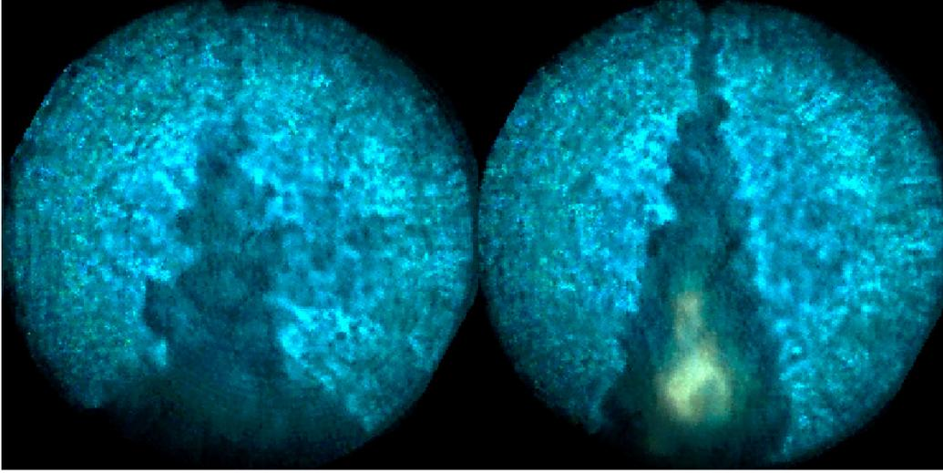
**Figure 3:** Neat ethanol injection, comparing injection timing and resultant soot formation
