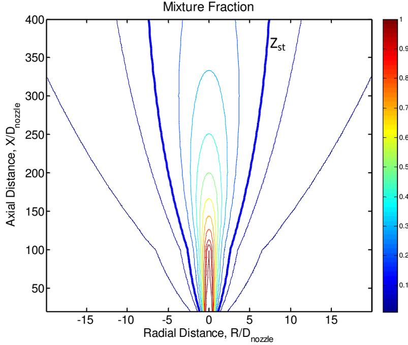
**Figure 4:** Model results showing mean mixture fraction within an ethanol injection
