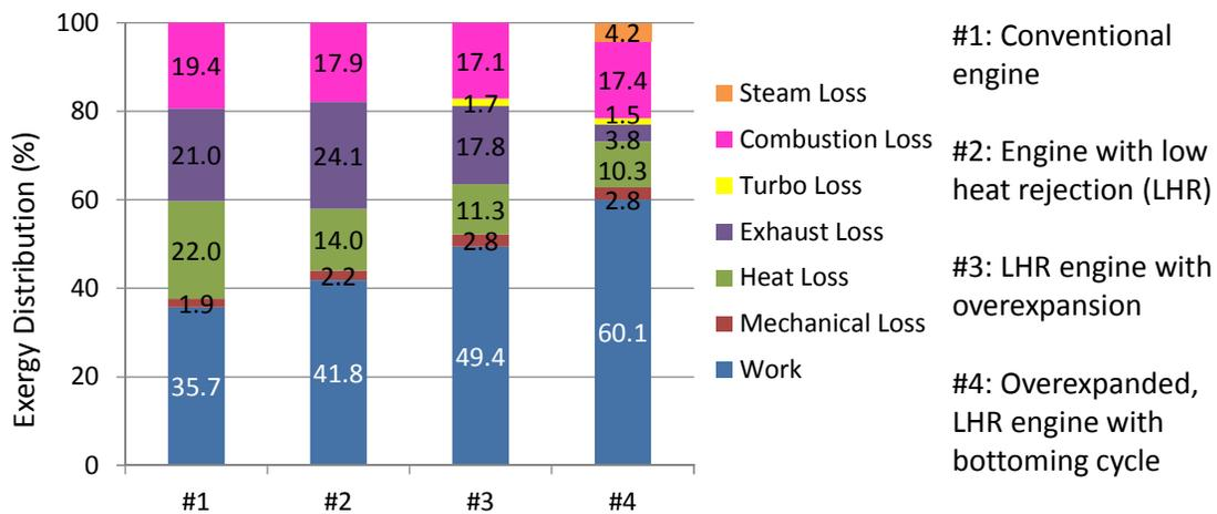
**Figure 7:** Fuel exergy distribution plots showing the increase in work output for low-heat-rejection strategies with exhaust enthalpy utilization
