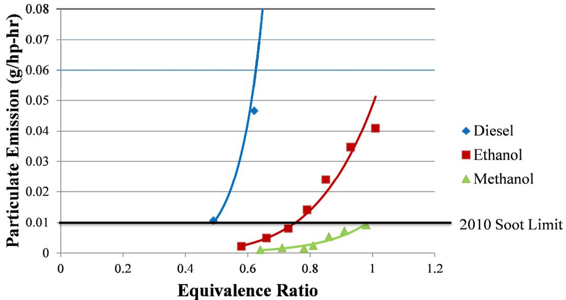
**Figure 6:** Smoke meter emission measurements from a single-cylinder reciprocating engine, comparing alcohol fuels and Diesel
