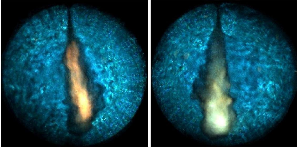
**Figure 1:** Comparison between methanol (left) and ethanol (right) injections
