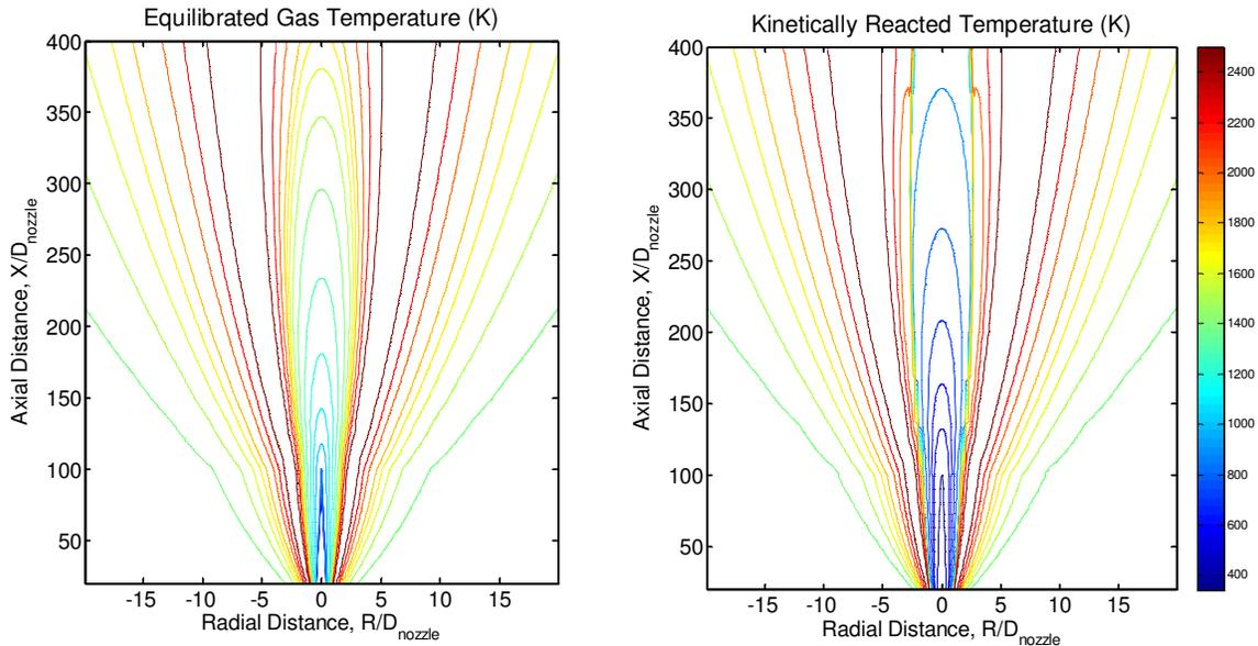
**Figure 5:** Model result comparing equilibrium temperature of the jet and the temperature obtained by applying a chemical reaction model
