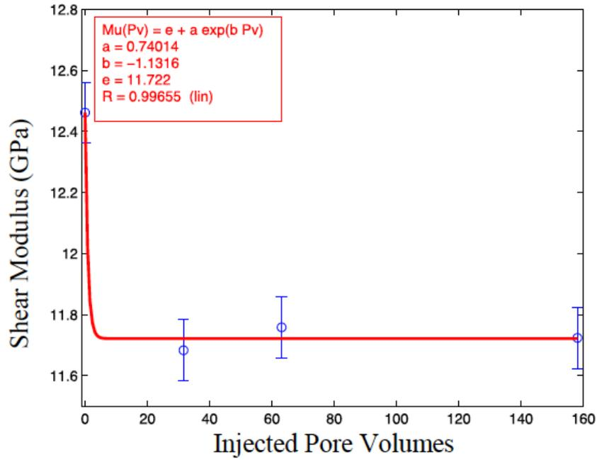
**Figure 9:** Shear modulus of the dry frame versus injected pore volumes for a differential pressure of 26 MPa.
