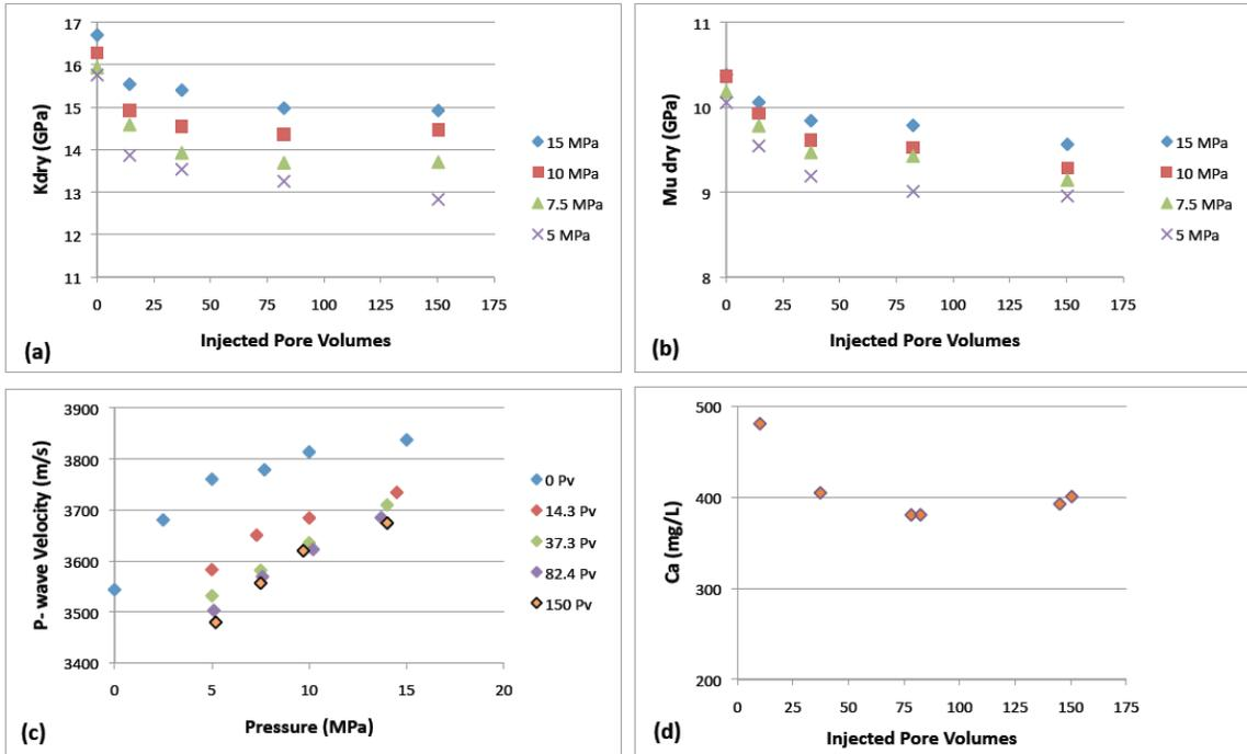
**Figure 1:** Variation of the bulk (a) and shear (b) moduli as functions of injected pore volumes. Data refer to micrite-rich grainstone from the MA formation and are color-coded as a function of confining pressure, (c) variation of P-wave velocity as a function of confining pressure. Data are color-coded as a function of the injected pore volumes, (d) variation of the concentration of the ion calcium in the collected fluid as function of the injected pore volumes.
