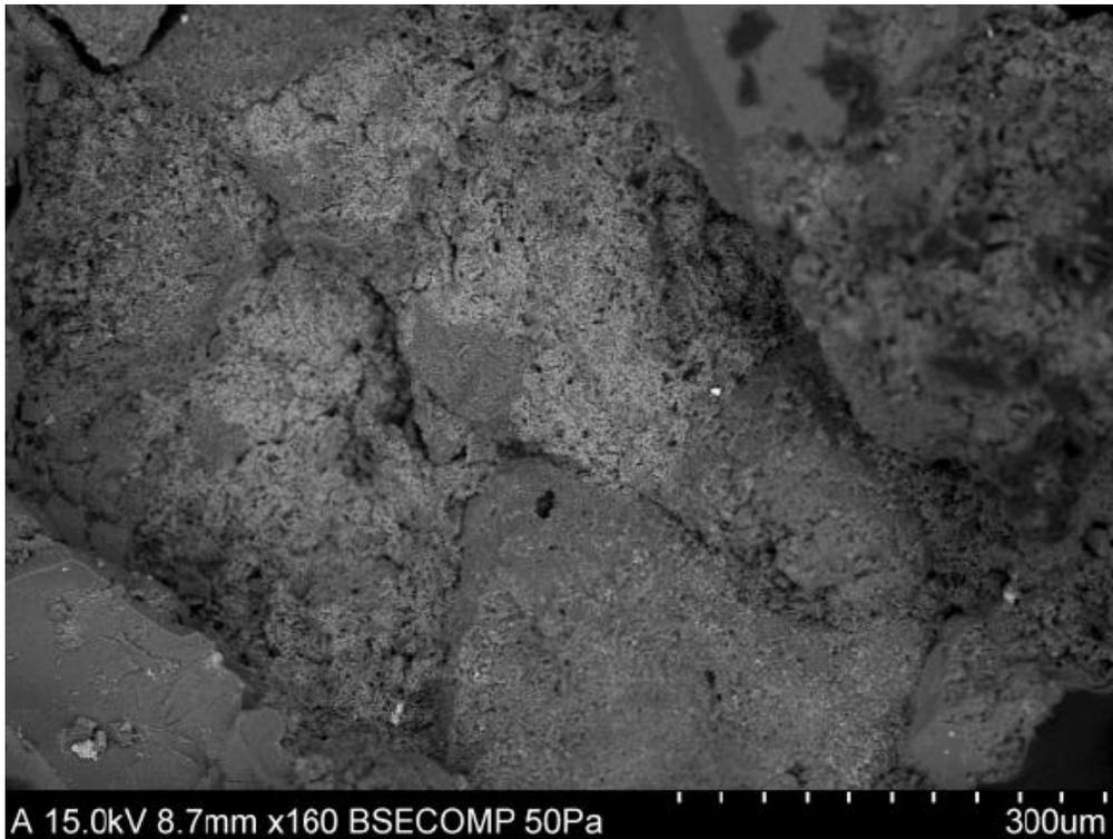
**Figure 11:** SEM image of the core plug before CO<sup>2</sup> rich brine.
