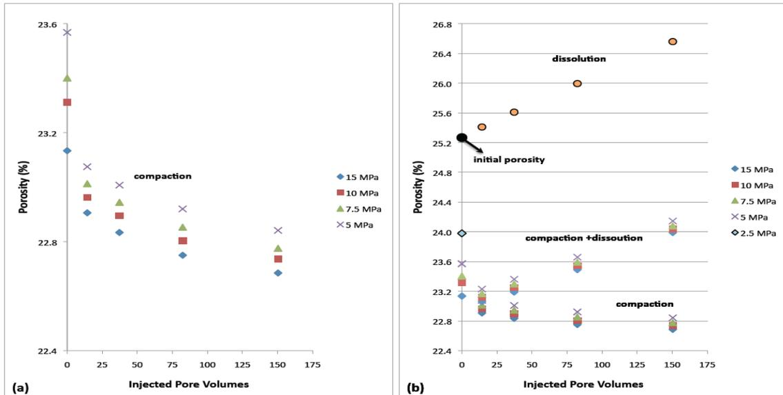
**Figure 2:** Variation of the porosity of the MA micrite-rich grainstone as a function of the injected pore volumes. The sample experiences a dissolution-driven compaction under the effect of the applied stress, eventually leading to porosity change.
