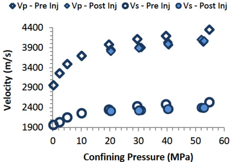
**Figure 6:** Compaction curves of the dried sample pre and post-injections. Pore pressure is zero.
