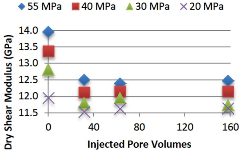
**Figure 7:** Shear modulus of the dry frame versus injected pore volumes colored by confining pressure.
