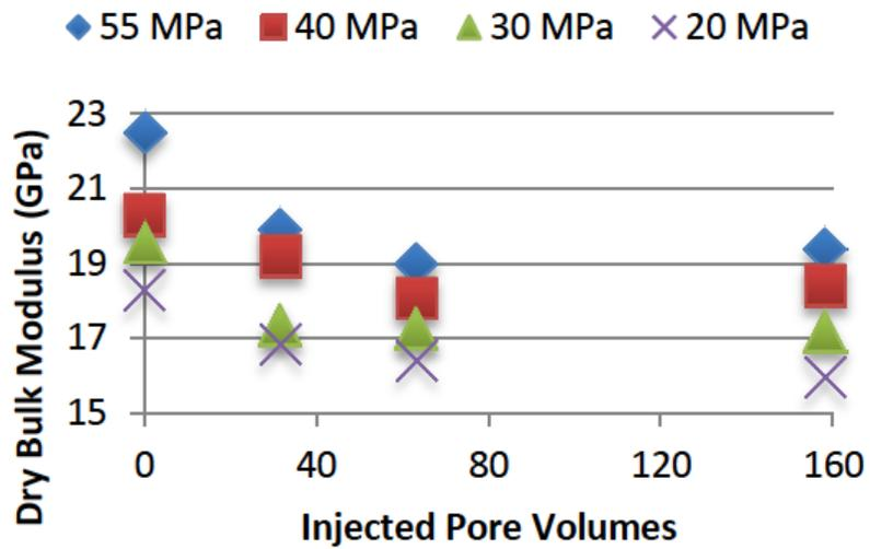
**Figure 8:** Bulk modulus of the dry frame versus injected pore volumes colored by confining pressure.
