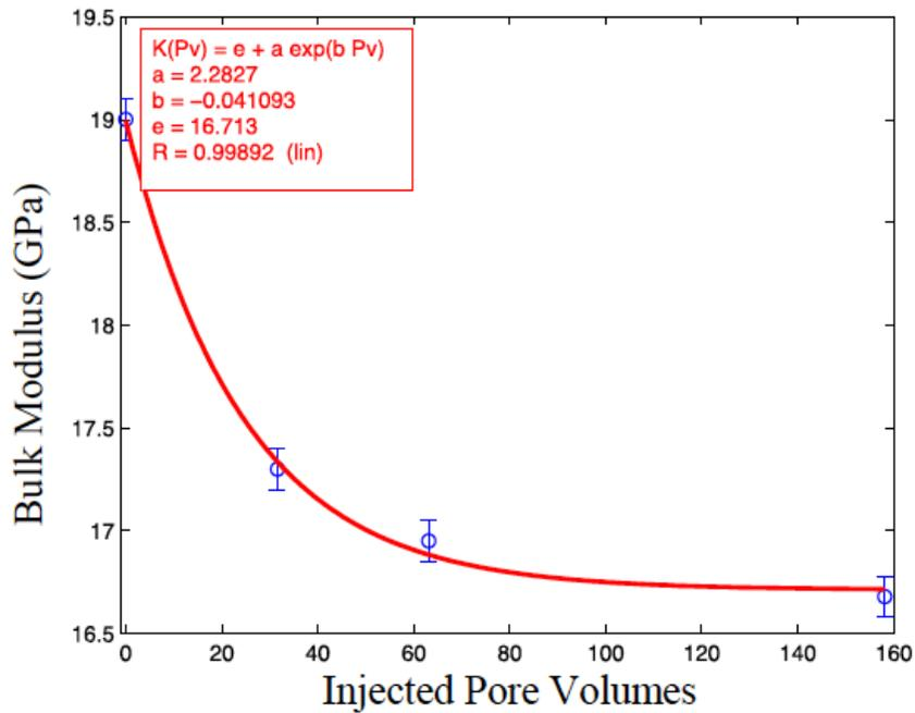
**Figure 10:** Bulk modulus of the dry frame versus injected pore volumes for a differential pressure of 26 MPa.
