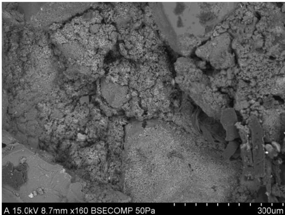
**Figure 12:** SEM image of the core plug after CO<sup>2</sup> rich brine.
