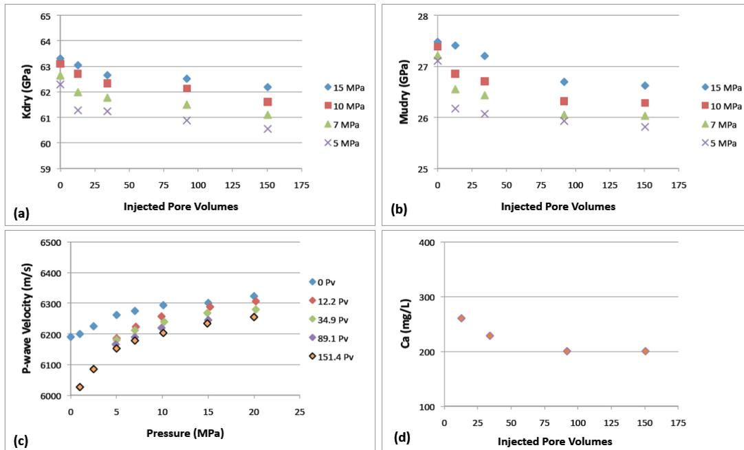
**Figure 3:** Variation of the bulk (a) and shear (b) moduli as functions of injected pore volumes. Data refer to a tight limestone from the MSA formation and are color-coded as functions of confining pressure, (c) variations of P-wave velocity as a function of confining pressure. Data are color-coded as functions of the injected pore volumes, (d) variation of the concentration of the ion calcium in the collected fluid as a function of the injected pore volumes.
