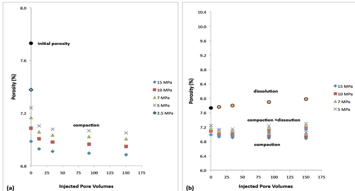
**Figure 4:** Variation of the porosity of the MSA tight limestone as a function of the injected pore volumes. The sample experiences a dissolution-driven compaction under the effect of the applied stress, eventually leading to porosity change.
