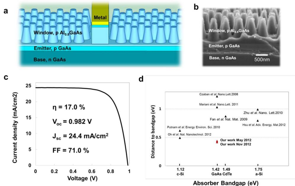
Figure 3. Overview of an AlGaAs/GaAs nanostructured window solar cell. (a) Schematic of the device structure. (b) SEM cross-section image of the solar cell active region with  $\text{Al}_{0.8}\text{GaAs}$  nanocone window layer. (c) 1 Sun J-V characterizations of the best sample. (d) band gap-voltage offset ( $E_g/q - V_{oc}$ ) for several published nanostructured solar cells with absorber materials of c-Si, GaAs, CdTe and a-Si.
