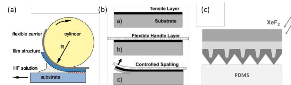
Figure 2. (a) A lift-off process to release GaAs solar cell layer by chemical etching.<sup>7</sup> (b) Scheme of Controlled spalling process.<sup>8</sup> (c) GaAs-Ge core-shell nanopylarids attached to PDMS superstrate in  $XeF_2$  gas etching.<sup>9</sup>
