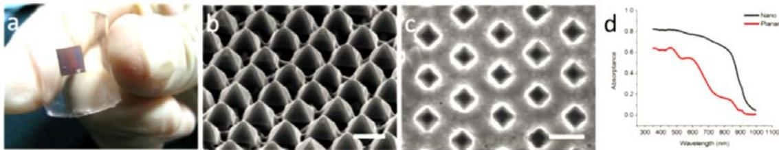
Figure 4. Characterizations of nanopyramid GaAs thin film. (a) Photograph of a bent 160nm-thick nanostructured GaAs film embedded in PDMS. SEM views of nanopyramid film (b) top surface and (c) back surface. Scale bars on (b) and (c) are 500nm. (d) Optical absorption spectra of nanopyramid film (black), planar film (red).
