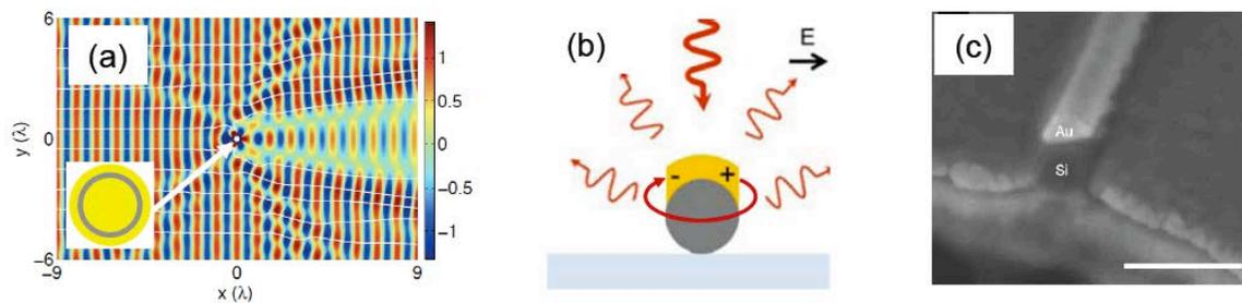
**Figure 6:** (a) A super-scattering nanowire consisting of metal (yellow) and dielectric (gray) regions in its cross-section as shown in the inset. (b) A light trapping scheme consisting of placing such super-scattering nanowires as shown in (a) onto a silicon substrate. (c) A scanning electron micrograph of a metal-coated silicon nanowire.
