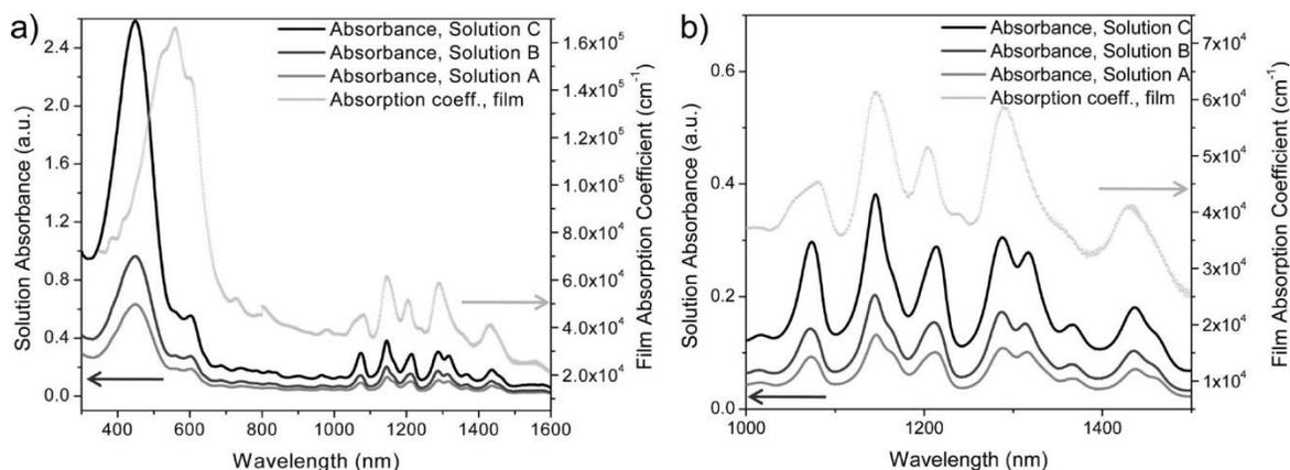
Figure 2 Absorption spectra of solutions and films of P3DDT sorted HiPco SWNTs
