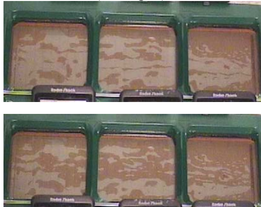
Figure 3: Examples of gas-water flow channels.
