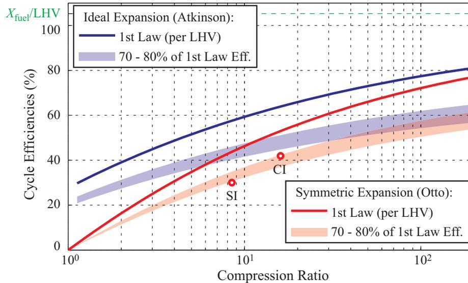
**Figure 3:** First law efficiencies vs. compression ratio for stoichiometric propane/air. As compression ratio increases,  $S_{gen}$  decreases and more exergy is transferred to work during expansion. As such, the Atkinson-cycle and Otto-cycle efficiencies begin to converge. The red and blue bands represent 70-80% of the first law efficiencies, which is representative of what current engines often achieve in practice after implementation efficiencies are included.
