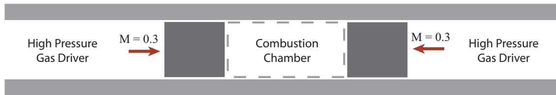
**Figure 4:** Basic concept of the extreme compression/expansion device. Two pistons are driven toward each other at high speed during the compression stroke. Fuel injection, autoignition, and combustion occur in the center region, driving each piston back toward its original position at high speed.
