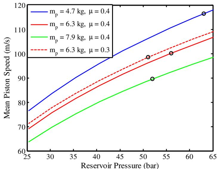
**Figure 7:** Mean piston speed as a function of initial reservoir pressure. The circles show the mean piston speed for the reservoir pressure that is associated with a 100:1 compression ratio based on Fig. 6.
