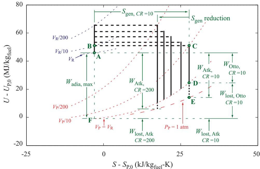
**Figure 2:** Ideal Otto and Atkinson cycles for stoichiometric propane/air on a  $U$ - $S$  diagram. Compression ratios shown include 10, 20, 50, 100, and 200:1. At a compression ratio of 200:1, the work lost due to combustion irreversibility can be reduced to one-half that from the 10:1 compression ratio case.
