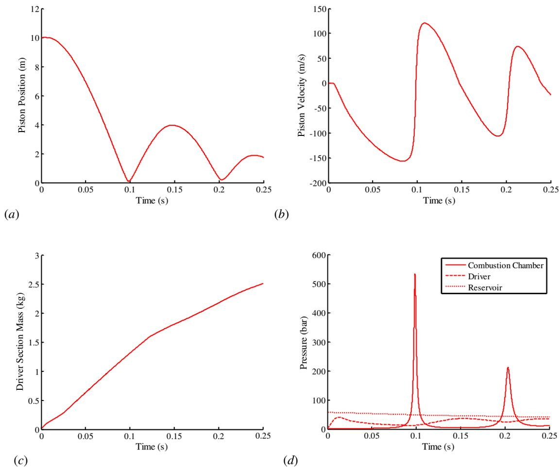
**Figure 8:** Dynamic simulation results for a single-piston system with a 6.3 kg piston and 56 bar, 0.18 m<sup>3</sup> gas reservoir. *a)* piston position *b)* piston velocity *c)* mass of air in the driver section and *d)* pressures as a function of time.
