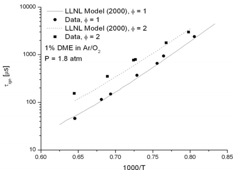
**Figure 6:** Ignition delay times for mixtures of 1% DME in Ar/O<sub>2</sub> and  $\phi = 1$  and 2 and comparison with the Curran, et al. model [6].
