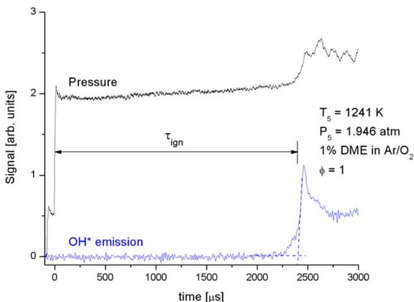
**Figure 5:** Example emission and pressure profiles during an ignition experiment. Reflected shock conditions: 1241 K, 1.946 atm, 1% DME in O<sub>2</sub>/argon,  $\phi = 1$ .
