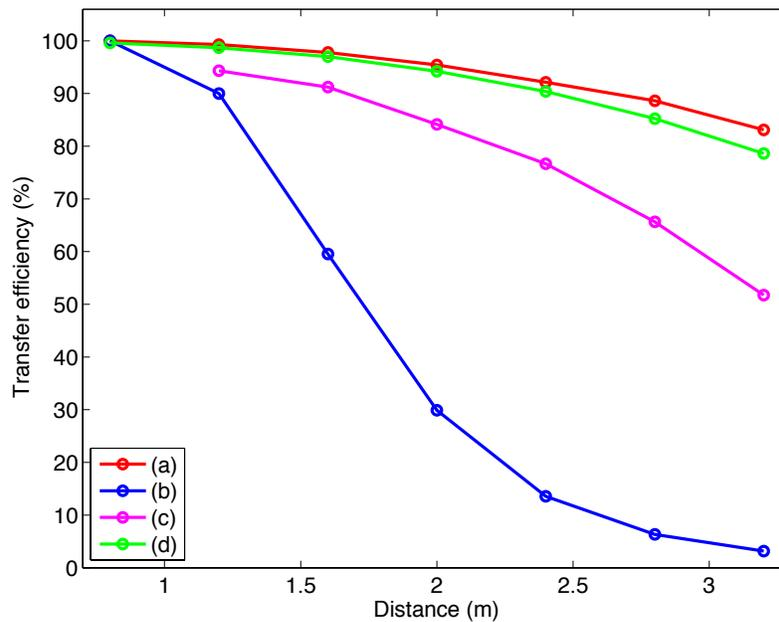
**Figure 4:** Transfer efficiencies as functions of the coil to coil distance for different structures shown in Fig. 3, assuming a working wavelength of  $30m$ .
