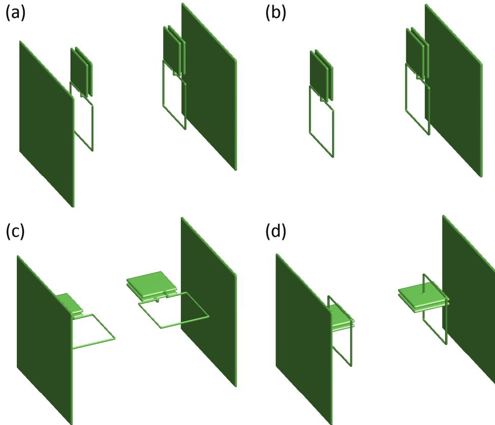
**Figure 3:** A variety of the resonator structures for the wireless energy transfer. (a) Our current optimal design with a “twisted” geometry. The distance between the coils  $\sim \lambda/15$ . Two metallic ground planes are placed near the system symmetrically. (b) Same system as (a) without the ground plane at the source coil side. (c) Same system as (a), but with the coil planes perpendicular to the ground planes. (d) Same system as (a) but with the capacitors at a different orientation.
