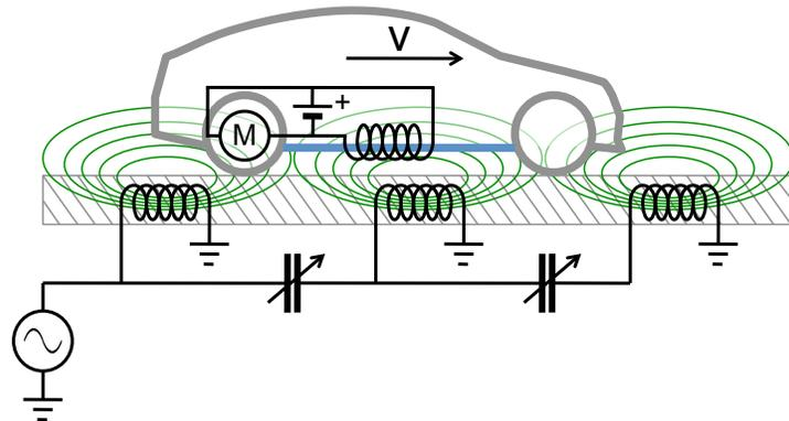
**Figure 2.** Magnetic Power Transmission to Vehicle on Highway.
