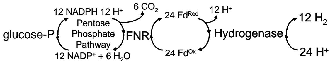
**Figure 1:** The pathway for conversion of chemical energy from glucose to hydrogen using the pentose phosphate pathway, ferredoxin NADP<sup>+</sup> reductase (FNR), a ferredoxin, and an [Fe-Fe] hydrogenase such as the CpI enzyme from *Clostridium pasteurianum* (*C.p.*).
