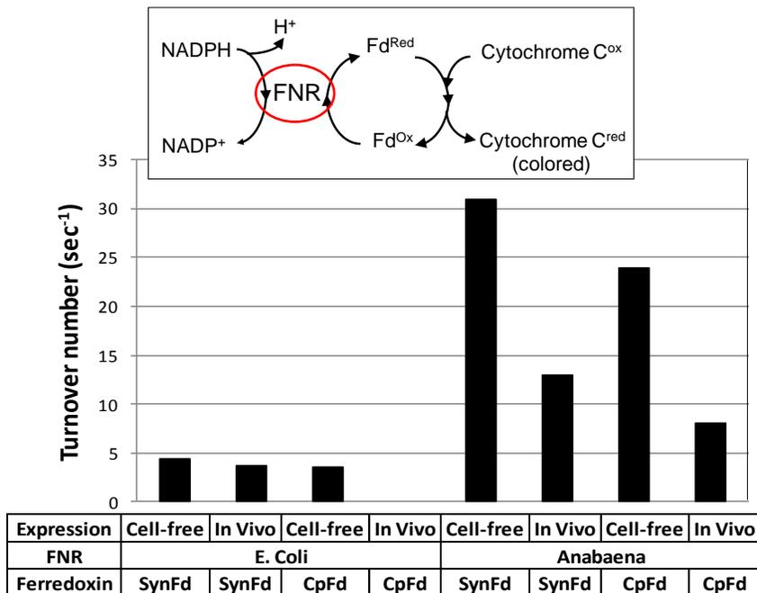
**Figure 2:** Characterization of the *E.coli* and *Anabaena* FNRs produced either *in vivo* by *E.coli* or by cell-free synthesis when coupled to ferredoxins either from *Synechocystis* (SynFd) or from *Clostridium pasteurianum* (CpFd). The upper inset indicates the assay format.
