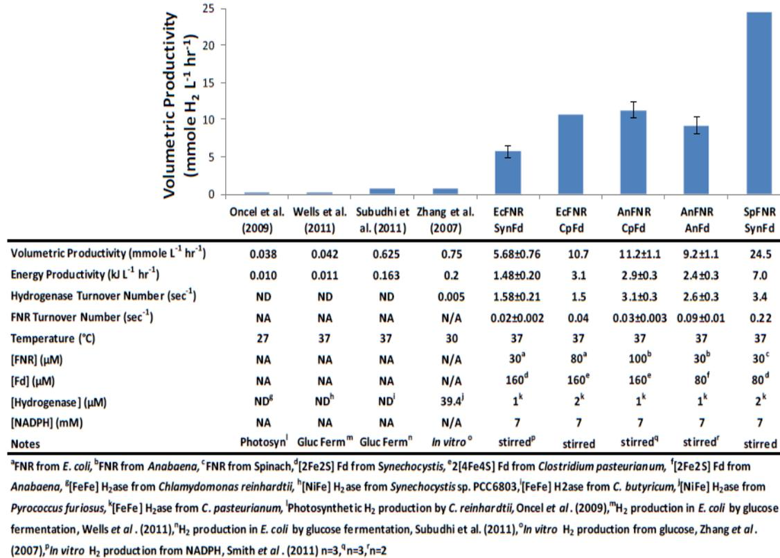
**Figure 3:** A comparison of the cell-free pathway performance versus state-of-the-art competing technologies. The table also indicates the measured turnover numbers of the hydrogenase and FNR enzymes using a variety of FNR's and ferredoxins with the Cpl [FeFe] hydrogenase.
