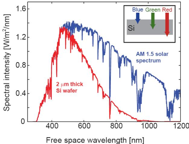
**Figure 1 | AM1.5 solar spectrum**, together with a graph that indicates the solar energy absorbed in a 2- $\mu\text{m}$ -thick crystalline Si film (assuming single-pass absorption and no reflection). Clearly, a large fraction of the incident light in the spectral range 600–1.100 nm is not absorbed in a thin crystalline Si solar cell.
