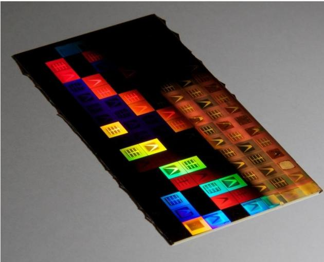
Photograph of plasmonic solar cells made in this GCEP project. An 8x16 array of ultra-thin amorphous silicon thin-film solar cells,  $4 \times 4 \text{ mm}^2$  each, is made in on a glass substrate patterned by soft imprint lithography. The different colors reflect the different light trapping geometries of the different cells.
