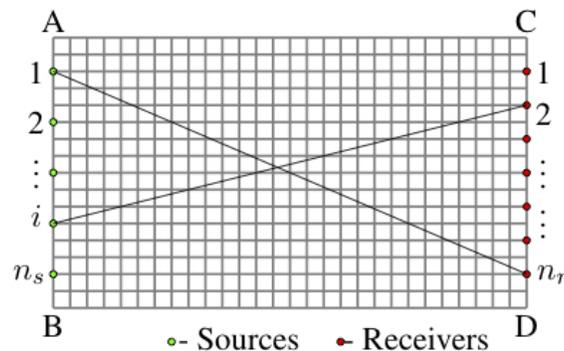
**Figure 2:** Cross section showing setup for seismic survey.
