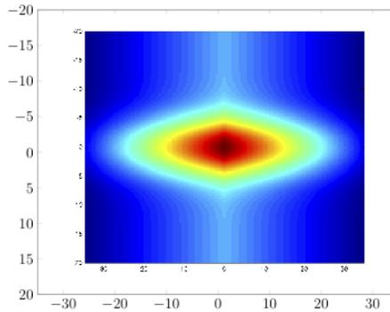
**Figure 3:** The image of slowness obtained based on a stochastic inverting method from cross-well seismic. Obtained for the  $10^6$ -node grid.
